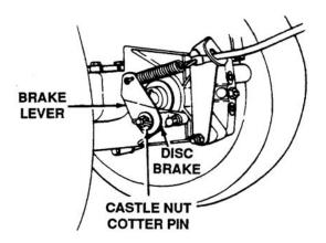
Figure 6-148. Brake Adjustment 700 and 800 Series Hydrostatic
