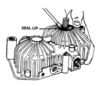
Figure 6-25. Oil Seal Removal
