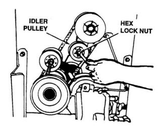
Figure 4-23. Idler Pulley Hex Lock Nut
