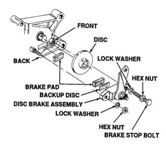
Figure 5-102. Disc Brake and Disc
