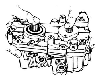
Figure 6-13. Removal of Center Section
