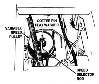
Figure 4-44. Location of Speed Selector Rod
