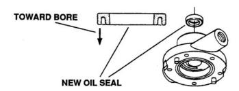
Figure 6-127. Oil Seal Installation
