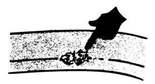
Figure 4-2. Belt Wear Due to Interference
