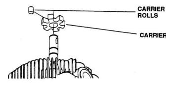
Figure 6-125. Installation of Carrier
