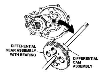
Figure 5-11. Differential Assembly
