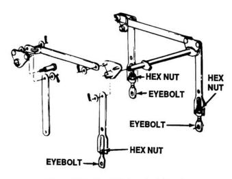
Figure 8-10. Deck Link Installation for 44-Inch Decks
