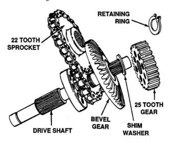
Figure 5-47. Removal of 25 Tooth Gear and Shim Washer
