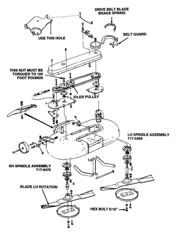
Figure 8-7. Model 931 44-Inch Rear Discharge Deck.
