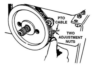
Figure 7-6. PTO Adjustment
