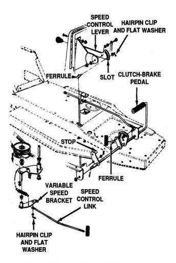
Figure 4-12. Speed Control Adjustment
