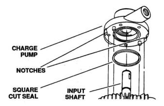
Figure 6-107. Removing Charge Pump Assembly
