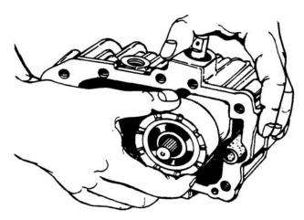
Figure 6-55. Installing Cylinder Block Kits in Housing
