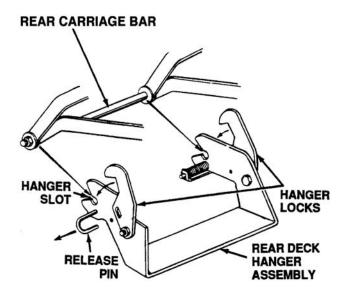
Figure 8-39. Pulling Release Pins
