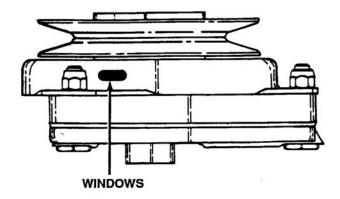
Figure 3-75. Checking Air Gap Setting
