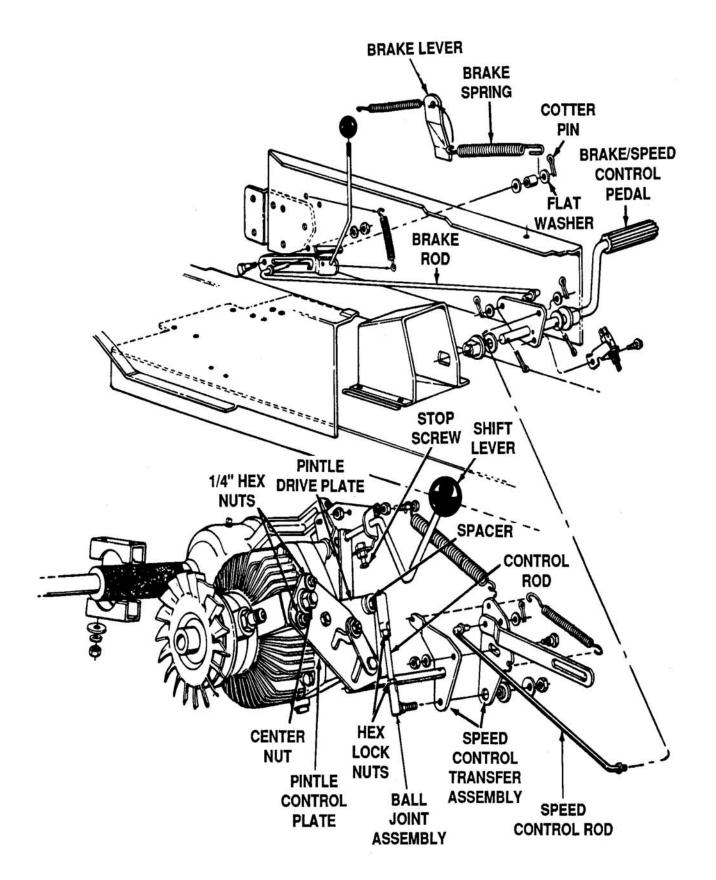
Figure 4-63. Adjusting Eaton Hydrostatic Control
