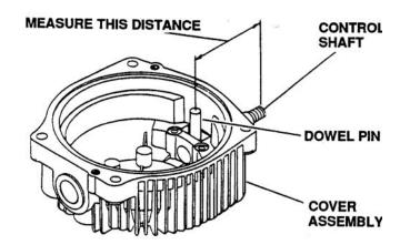
Figure 6-112. Removal of Control Shaft
