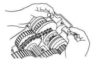
Figure 5-58. Placing Pins in Housing
