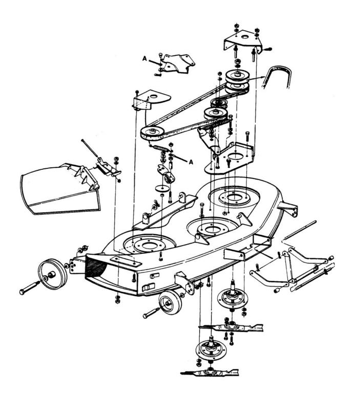
Figure 8-20. Models 806, 846, and Series 800 "H" Side Discharge Deck
