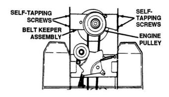
Figure 4-55. Belt Keeper Assembly
