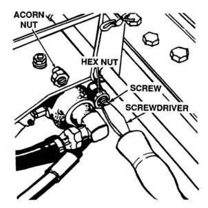
Figure 7-5. Adjusting Hydraulic Lift Valve
