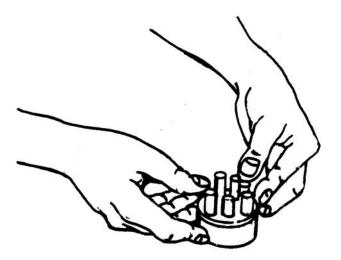
Figure 6-54. Checking Movement of Pistons in Bores
