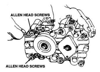
Figure 6-12. Location of Allen Head Screws
