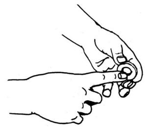
Figure 6-67. Greasing Oil Seal Lip
