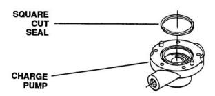
Figure 6-128. Installing Square Cut Seal
