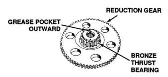
Figure 5-108. Reduction Gear Inspection and Replacement
