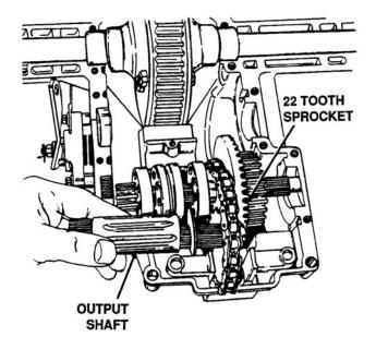
Figure 5-44. Removal of Output Shaft
