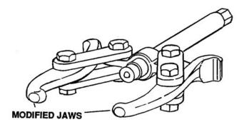
Figure 6-106. 2-Jaw Bearing Puller
