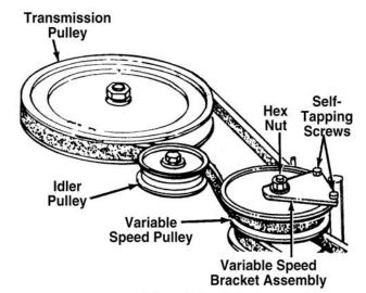
Figure 4-41. Front Drive Belt Removal
