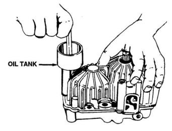
Figure 6-11. Oil Tank Removal
