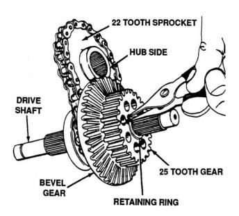
Figure 5-46. Removing Retaining Ring
