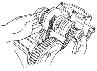
Figure 5-55. Installing Gear Cluster and Bearings
