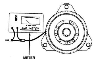
Figure 3-74. Measuring Clutch Current Draw
