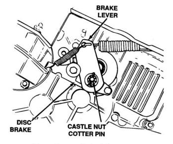
Figure 4-69. Brake Adjustment
