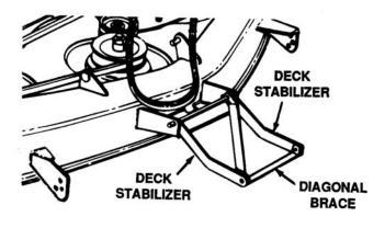
Figure 8-23. Deck Stabilizers and Diagonal Brace
