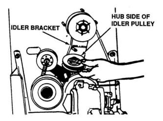
Figure 4-25. Reassembly of Idler Pulley
