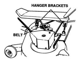
Figure 8-31. Attaching Hanger Brackets
