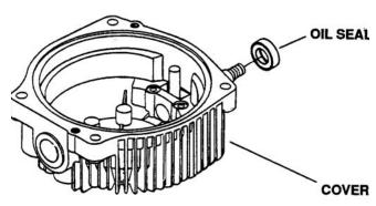
Figure 6-117. Installing Oil Seal
