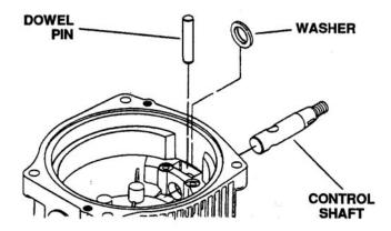
Figure 6-115. Install Control Shaft and Washer
