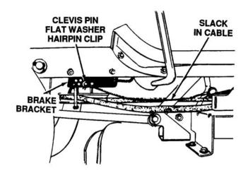
Figure 8-5. Connecting the Brake Cable
