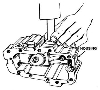
Figure 6-38. Pressing Journal Bearing Into Housing
