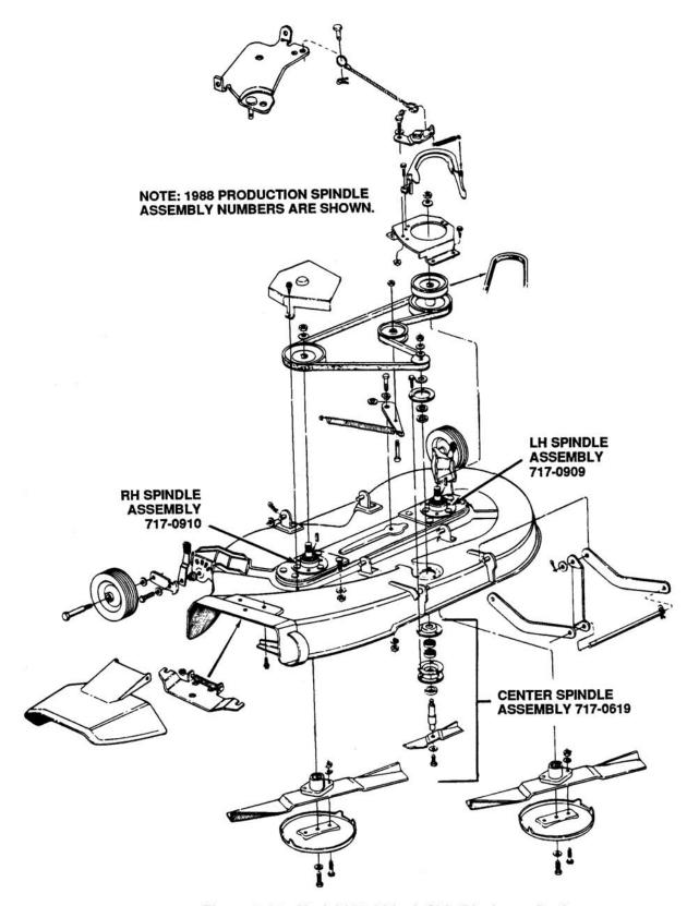
Figure 8-17. Model 935 44-Inch Side Discharge Deck
