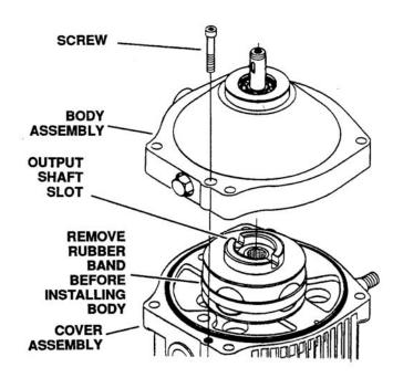
Figure 6-137. Body Installation
