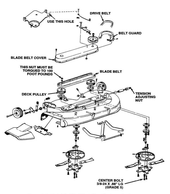
Figure 8-18. Model 194-935 44-Inch Side Discharge Deck
