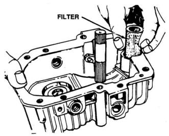
Figure 6-23. Removal of Filter
