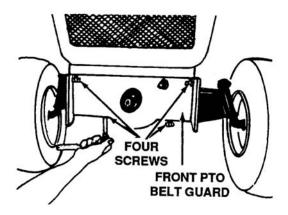
Figure 7-7. Removing PTO Belt Guard Assembly
