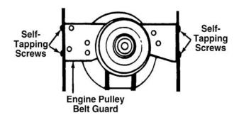
Figure 4-42. Engine Pulley Belt Guard
