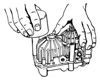
Figure 6-77. Installing Cap Onto Housing
