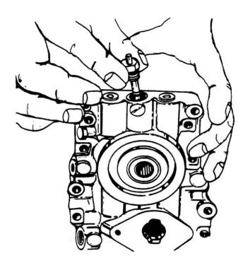
Figure 6-74. Installation of Bypass Valve
