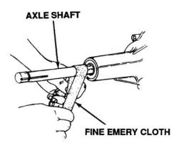
Figure 5-103. Cleaning Axle Shaft
