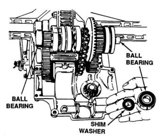
Figure 5-35. Removal of Bearings and Shim Washers
