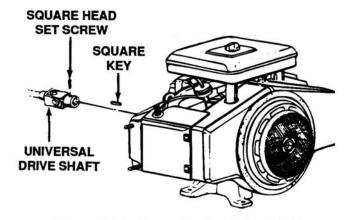
Figure 7-11. Removing the Drive Shaft
