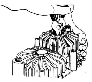
Figure 6-46. Installing Retaining Ring
