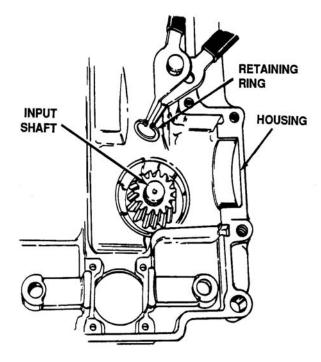
Figure 5-51. Removal of Retaining Ring
