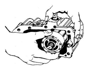
Figure 6-17. Removing Pump and Motor
