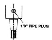
Figure 6-114. Install Pipe Plug
