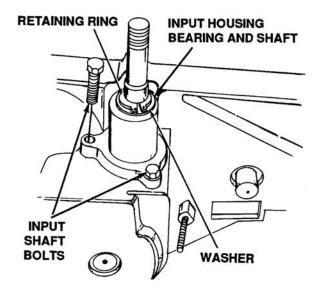
Figure 5-101. Input Housing Bearing and Shaft
