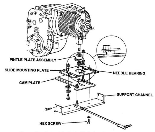
Figure 7-3. Hydrostatic Control Adjustment
