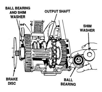
Figure 5-41. Removing Ball Bearings and Shim Washers
