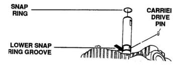
Figure 6-122. Installing Lower Snap Ring
