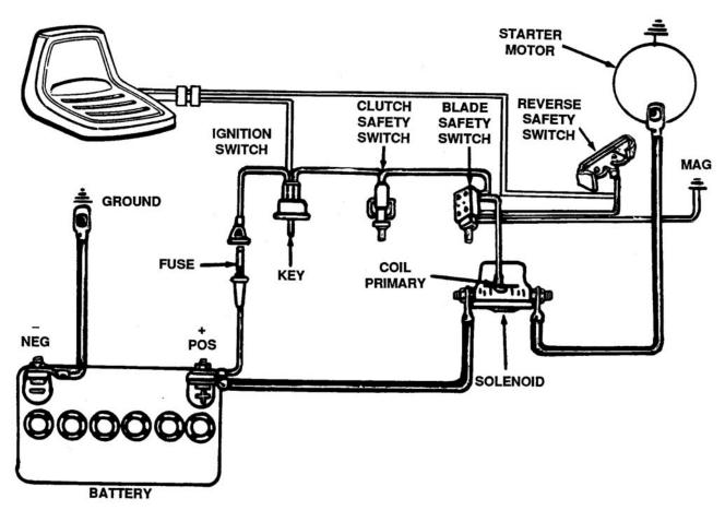
Figure 3-8. Typical Electric Start System.
