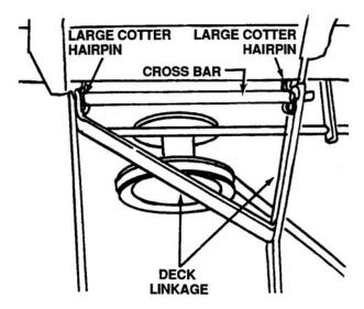
Figure 8-13. Disassemble/Reassemble Cross Bar
