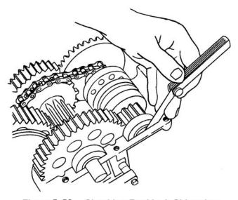
Figure 5-56. Checking Backlash Shimming
