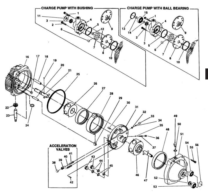
Figure 6-81. Model 11 Transmission
