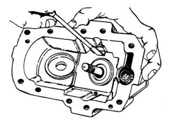
Figure 6-49. Install Swashplate
