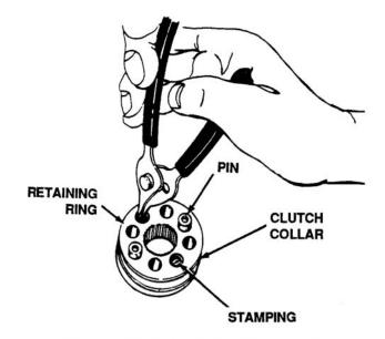
Figure 5-37. Clutch Collar Disassembly
