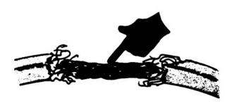
Figure 4-4. Belt Damage Due to Shock Load
