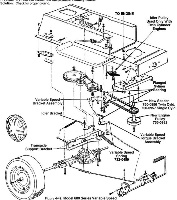
In many cases, we have found if speeds cannot be obtained after checking major components and performing a variable speed adjustment, the problem usually is between the variable speed bracket assembly and torque bracket assembly not fully pivoting.
