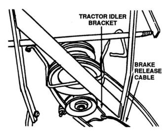
Figure 8-14. Securing Brake Release Cable
