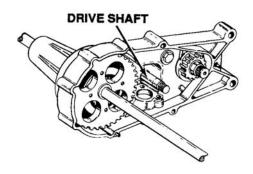
Figure 5-107. Reduction Gear Removal
