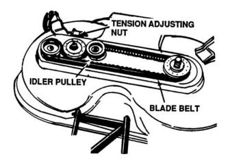
Figure 8-16. Removing Blade Belt
