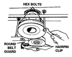
Figure 8-29. Removing Belt Guard
