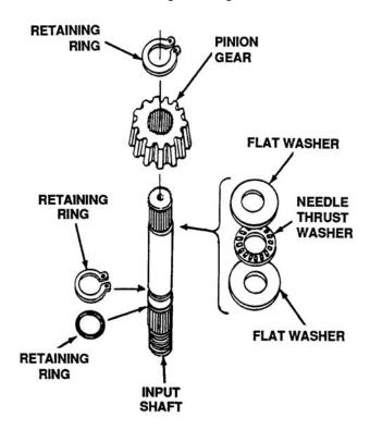
Figure 5-52. Input Shaft Thrust Washer
