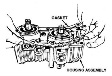
Figure 6-14. Removing Gasket
