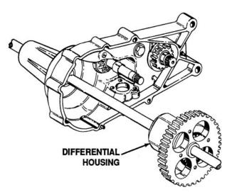
Figure 5-109. Differential Removal
