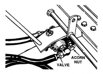
Figure 7-4. Location of Hydraulic Lift Valve
