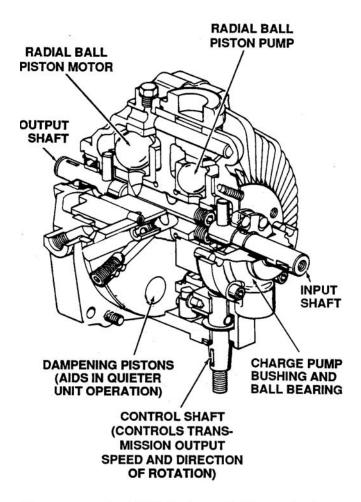
Figure 6-78. Model 11 Hydrostatic Transmission
