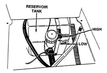
Figure 4-71. Checking Hydrostatic Oil Level
