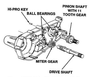
Figure 5-111. Pinion Shaft With 11 Tooth Gear Removal
