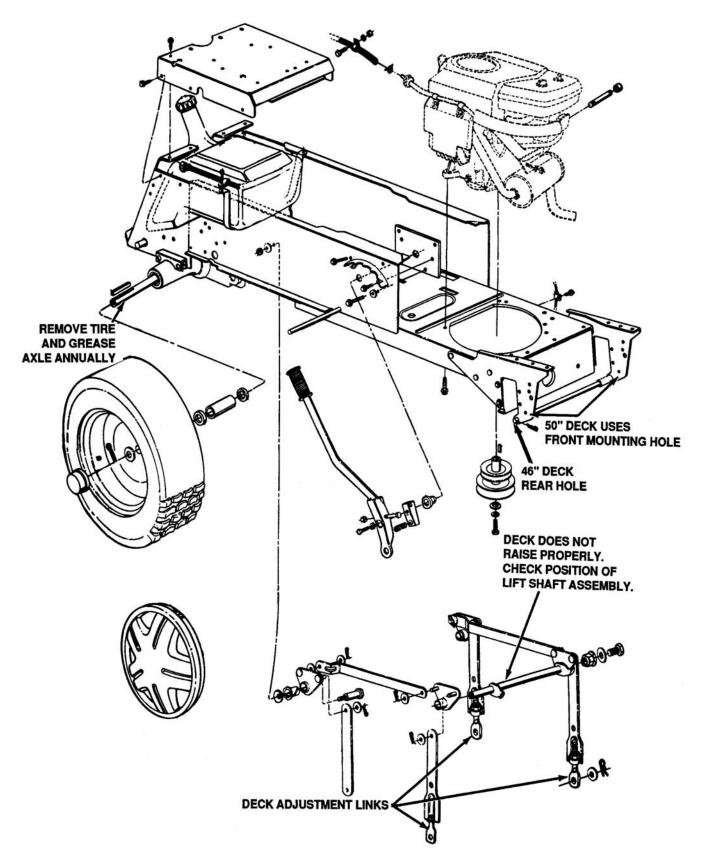
Figure 8-8. 44-Inch, 46-Inch, and "P" 50-Inch Deck Mounting
