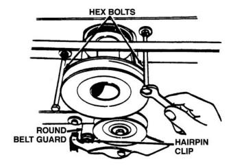
Figure 8-22. Removing Belt Guard
