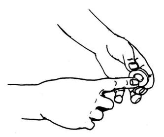
Figure 6-43. Greasing Oil Seal Lip
