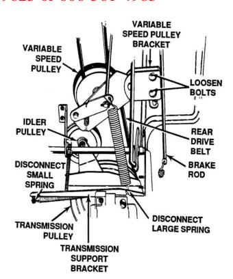
Figure 4-18. Location of Pulleys
