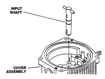
Figure 6-110. Removing Input Shaft From Cover Assembly
