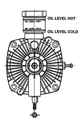
Figure 6-4. Reservoir/Expansion Tank
