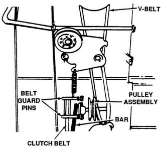
Figure 4-61. Removing Belt From Pulley Assembly
