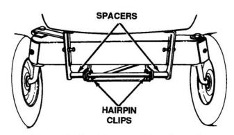
Figure 8-32. Disassembling Cross Bar
