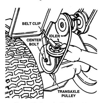
Figure 4-62. Removing Idler Assembly
