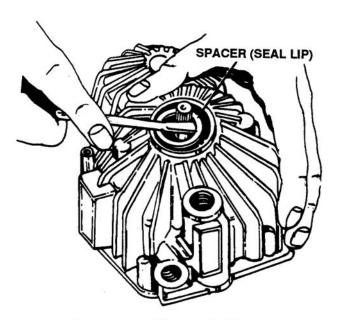
Figure 6-26. Removal of Spacer
