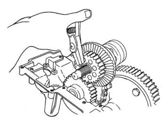
Figure 5-38. Removal of High Gear Snap Ring
