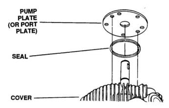
Figure 6-120. Installing Square Cut Seal
