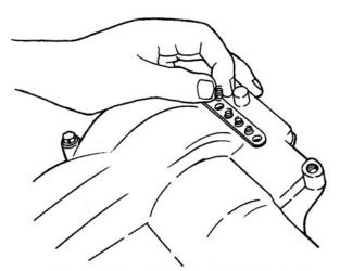
Figure 5-62. Installing Detent Springs
