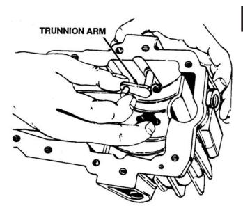
Figure 6-28. Removal of Trunnion Arm
