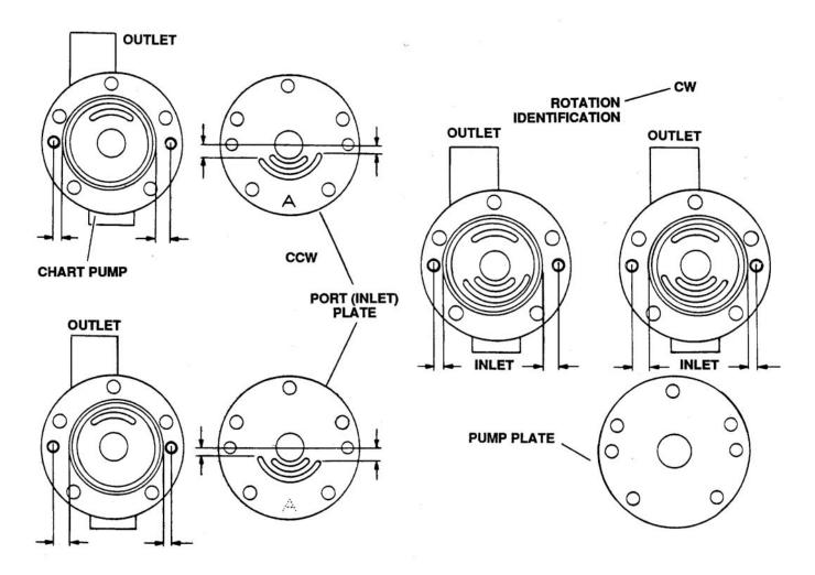
Figure 6-121. Installing Pump Plate
