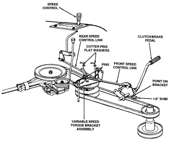
Figure 4-9. Two Speed Transmission
