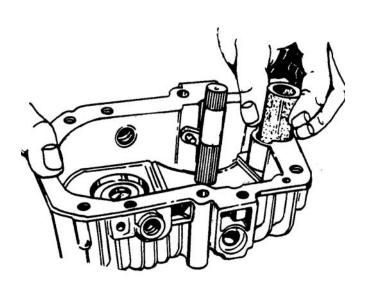
Figure 6-47. Installing Filter
