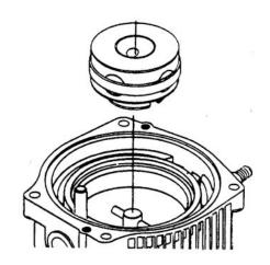
Figure 6-133. Pump Rotor Installation
