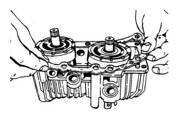
Figure 6-61. Installing Gasket
