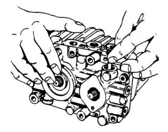
Figure 6-71. Installing Ball, Spring and Plug
