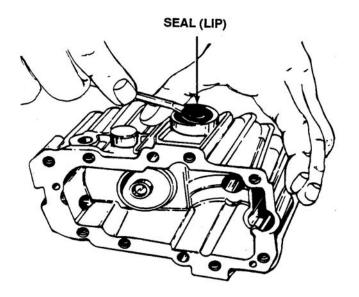
Figure 6-29. Oil Seal Removal
