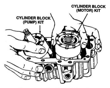
Figure 6-56. Checking Rotation of Cylinder Block Kits
