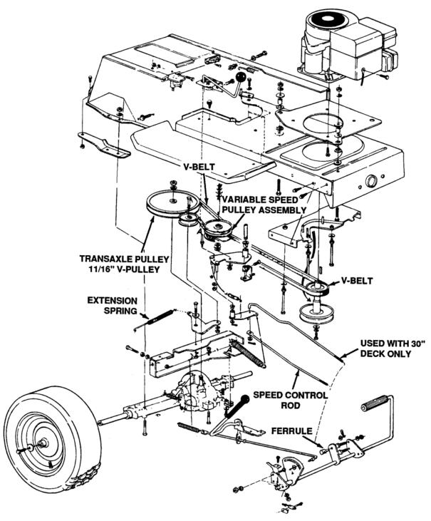
Figure 4-27. Variable Speed Drive System for 600 and 700 Series
