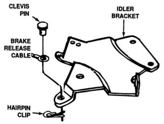
Figure 8-26. Tractor Idler Bracket
