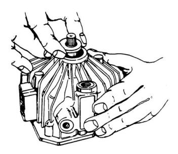
Figure 6-42. Installing Spacer
