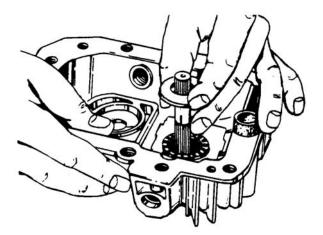
Figure 6-50. Installing Thrust Plate and Thrust Roller
