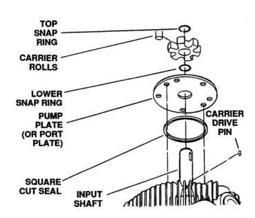
Figure 6-104. Input Shaft Disassembly
