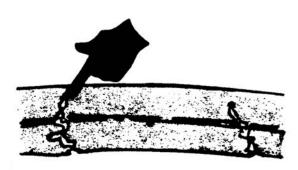
Figure 4-5. Belt Damage Due to Flex Failure
