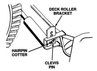
Figure 8-38. Deck Roller Bracket
