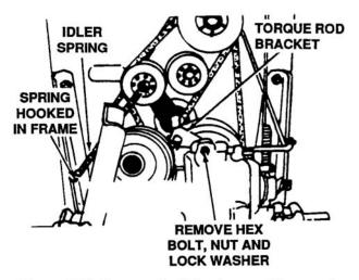
Figure 4-19. Torque Rod Bracket and Transaxle
