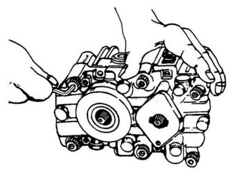
Figure 6-63. Location of Allen Head Screws
