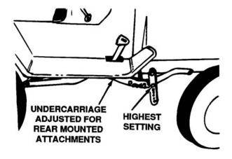
Figure 7-10. Undercarriage Lock Raised Position
