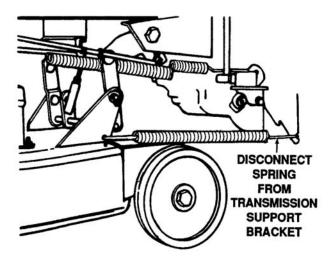
Figure 4-45. Transmission Support Bracket
