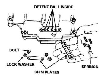
Figure 5-30. Removing Shim Plates
