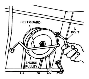
Figure 4-74. Releasing Belt Guard
