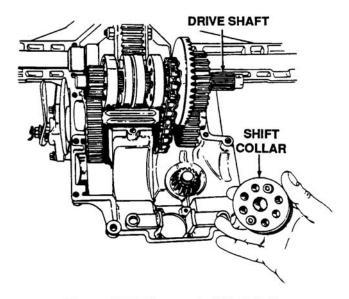
Figure 5-36. Removal of Shift Collar
