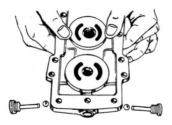
Figure 6-33. Ball and Spring Removal
