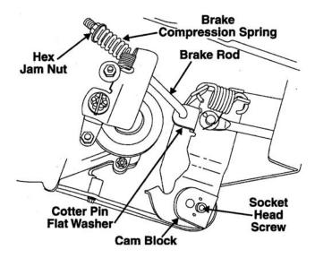
Figure 6-151. Brake Adjustment
