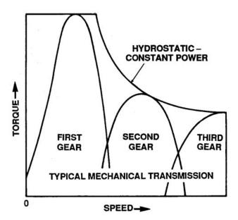
Figure 6-1. Hydrostatic/Mechanical Transmission Performance Graph
