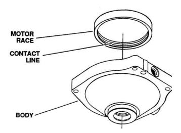
Figure 6-84. Inspecting Motor Race
