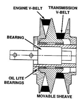
Figure 4-11. Vertical Variable Speed Drive Pulley
