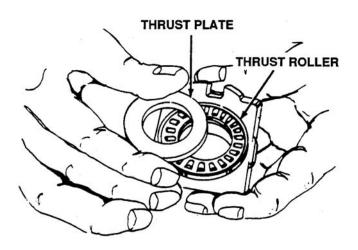
Figure 6-21. Thrust Plate and Thrust Roller
