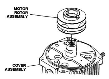
Figure 6-85. Removing Motor Rotor Assembly
