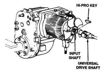
Figure 7-12. Drive Shaft Removal
