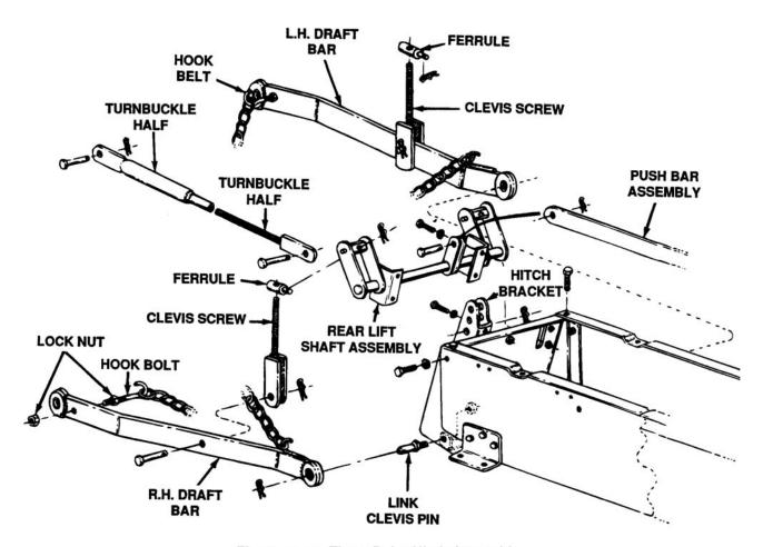
Figure 7-13. Three Point Hitch Assembly
