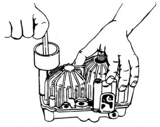
Figure 6-76. Installing Oil Tank Assembly
