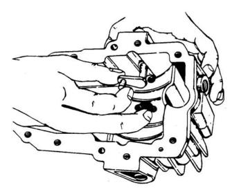
Figure 6-39. Installing Trunnion Arm
