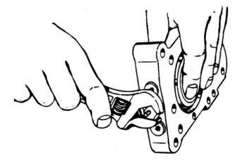
Figure 6-75. Tightening Plug
