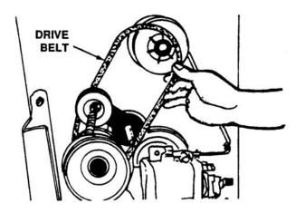
Figure 4-24. Removing Drive V-Belt
