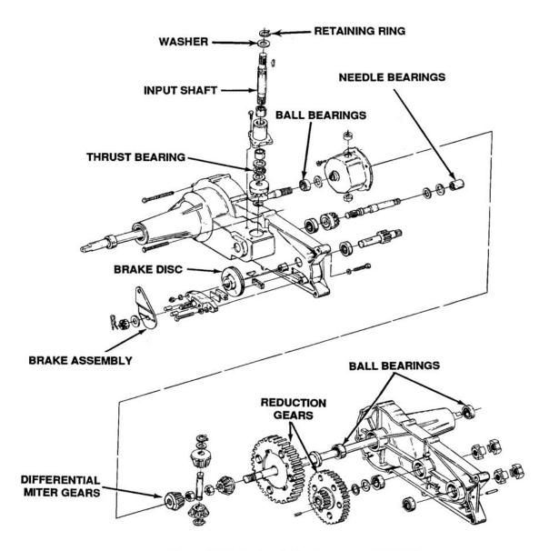
Figure 5-98. Hydrostatic Transaxle 717-0950
