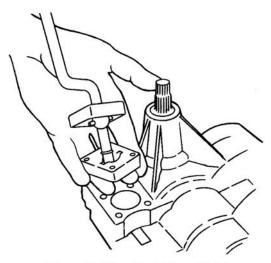
Figure 5-64. Installing Shifter
