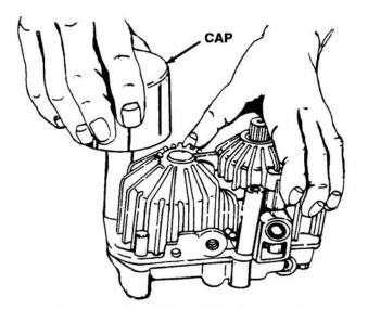
Figure 6-10. Oil Tank Cap Removal
