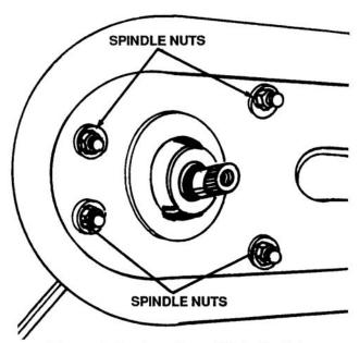
Figure 8-19. Location of Spindle Nuts
