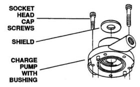
Figure 6-101. Removing Charge Pump
