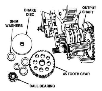
Figure 5-42. Removal of 45 Tooth Gear
