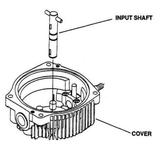
Figure 6-118. Installing Input Shaft
