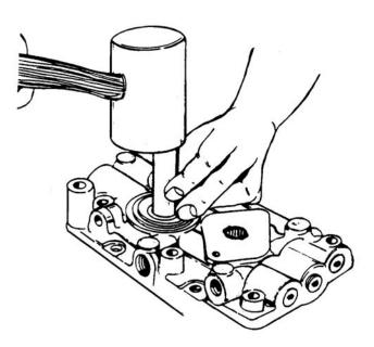
Figure 6-66. Pressing Seal Into Center Section
