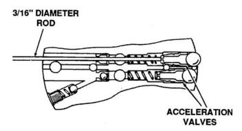
Figure 6-96. Removing Acceleration Valve Body
