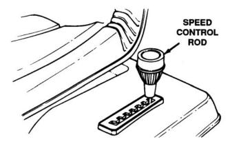
Figure 4-58. Speed Control Lever
