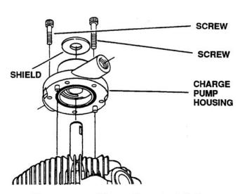
Figure 6-129. Charge Pump Installation
