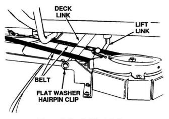
Figure 8-2. Belt Installation
