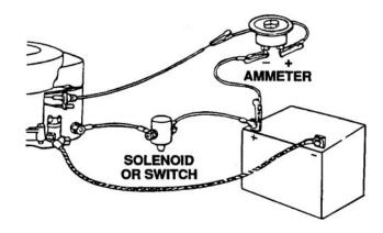
Figure 2-8. Alternator Charging Output
