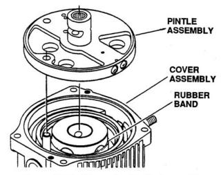
Figure 6-87. Removing Pintle Assembly
