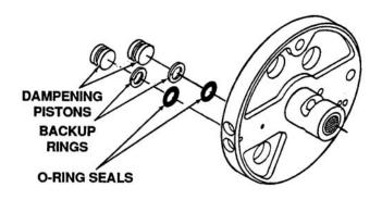
Figure 6-90. Removing Dampening Pistons
