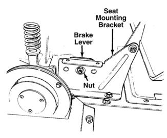
Figure 4-40. Brake Adjustment
