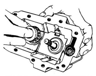
Figure 6-52. Replacing Thrust Ball Bearing
