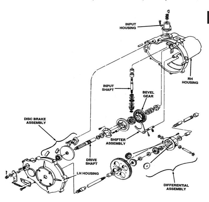
Figure 5-1. Heavy Duty Single Speed Transaxle
