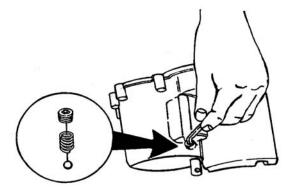
Figure 5-14. Removing Detent Spring and Ball
