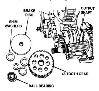
Figure 5-43. Removal of 45 Tooth Gear
