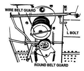
Figure 8-11. Removing Round Belt Keeper
