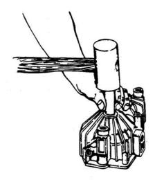
Figure 6-69. Pressing Seal Into Housing
