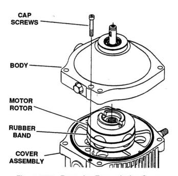
Figure 6-82. Removing Transmission Cover
