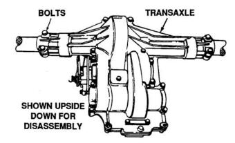
Figure 5-31. Removing Bolts From Transaxle
