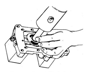
Figure 6-37. Removal of Needle Bearing 6-3.12 Assembly of Sundstrand BDU-10S.
