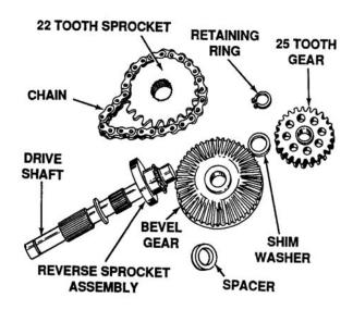
Figure 5-48. Drive Shaft Disassembly
