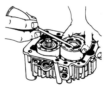
Figure 6-60. Lubricating Cylinder Block
