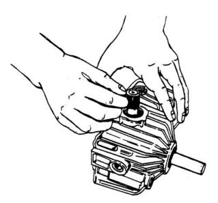
Figure 6-68. Covering Trunnion Arm With Tape
