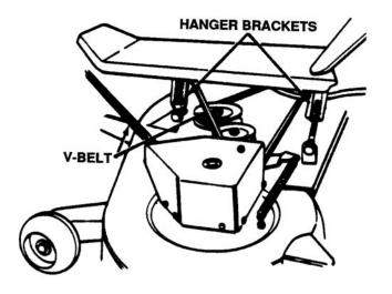
Figure 8-24. Attaching Hanger Brackets
