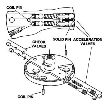
Figure 6-94. Removing Acceleration Valves
