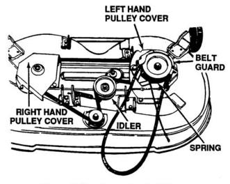
Figure 8-6. Removing Belt Guard
