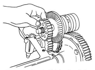
Figure 5-39. Removing High Gear From Shaft
