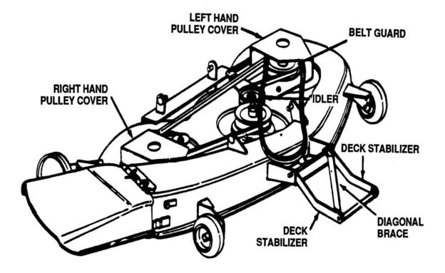
Figure 8-27. Removing Pulley Covers
