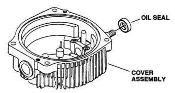
Figure 6-111. Removing Oil Seal From Cover
