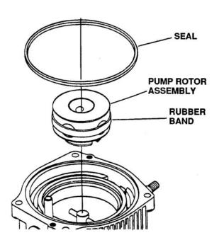
Figure 6-98. Removing Pump Rotor Assembly
