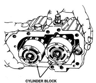
Figure 6-16. Cylinder Block
