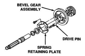
Figure 5-16. Removing Spring Retaining Plate
