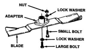
Figure 8-35. Cutting Blade
