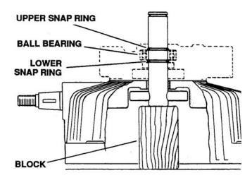
Figure 6-130. Ball Bearing Installation
