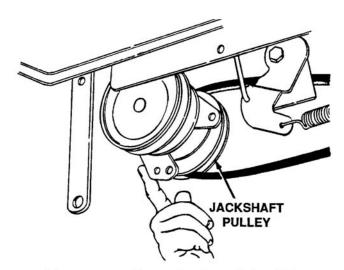
Figure 4-73. Removing Front Drive Belt From Jackshaft Pulley
