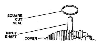
Figure 6-102. Removing Square Cut Seal
