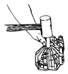
Figure 6-41. Pressing Shaft Into Housing
