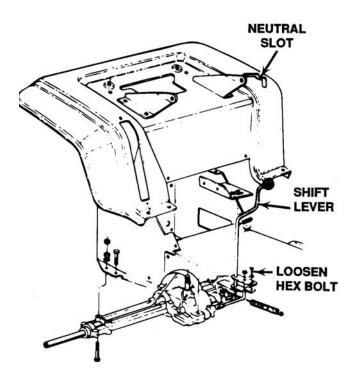
Figure 4-13. Adjusting Shift Lever to Neutral
