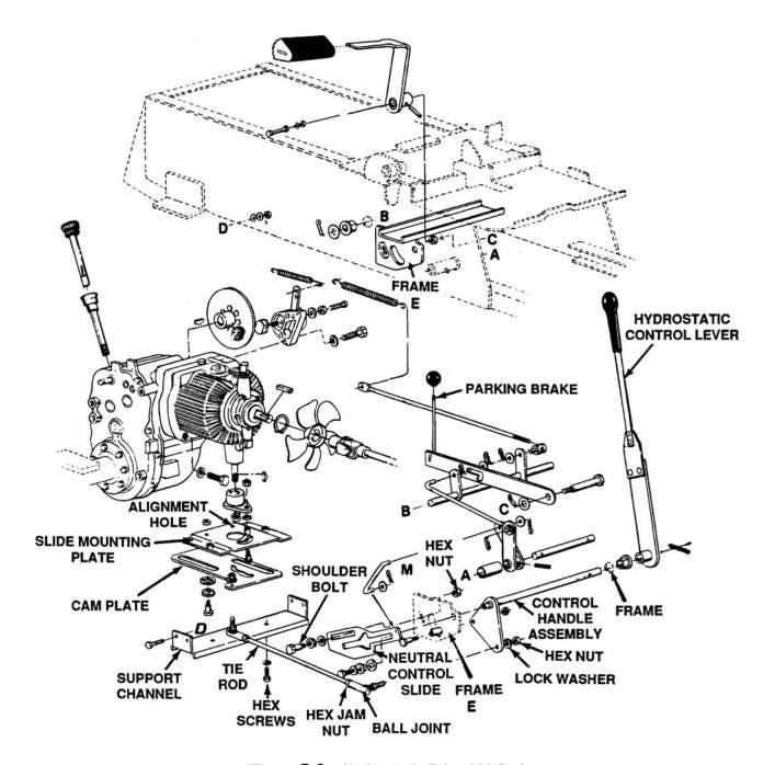
Figure 7-2. Hydrostatic Drive 900 Series
