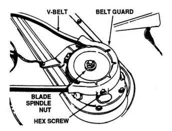
Figure 8-15. Removal and Replacement of Deck Belt
