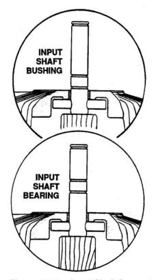
Figure 6-119. Input Shaft Support
