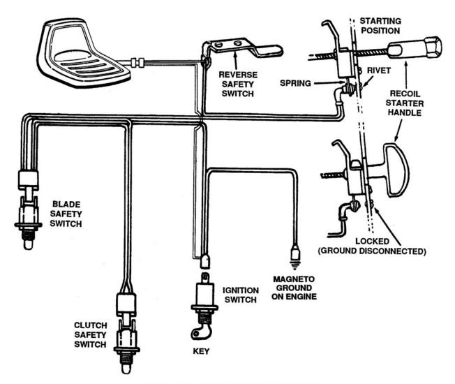
Figure 3-9. Typical Recoil Start System
