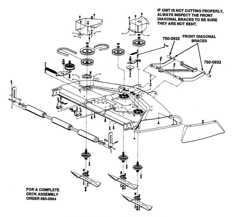
Figure 8-28. Model Series 800 "P" 50-Inch Deck
