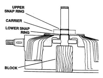
Figure 6-126. Installing Upper Snap Ring
