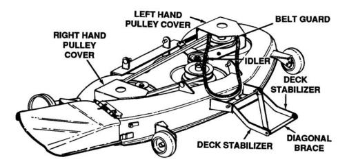
Figure 8-34. Removing Pulley Covers
