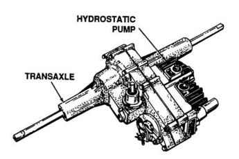
Figure 5-99. Transaxle and Pump
