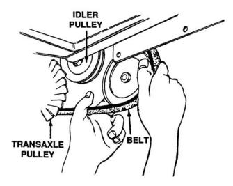
Figure 4-72. Removing Rear Drive Belt
