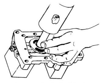
Figure 6-59. Pressing Needle Bearing Into Center Section
