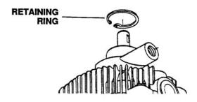
Figure 6-131. Installing Large Retaining Ring
