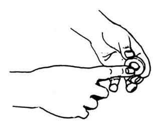
Figure 6-64. Greasing Oil Seal Lip
