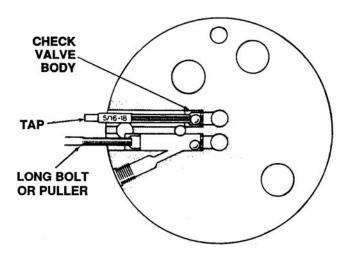
Figure 6-93. Removing Check Valve Bodies
