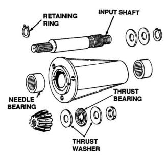
Figure 5-3. Disassembly of Input Shaft
