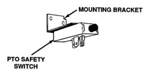
Figure 3-2. Mounting Bracket.
