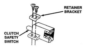
Figure 3-5. Retainer Bracket.
