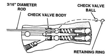
Figure 6-95. Removing Check Valve Ball
