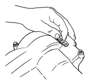
Figure 5-61. Installing Detent Balls
