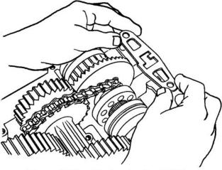
Figure 5-59. Placing Lockout Plate
