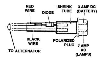
Figure 2-6. Dual Circuit
