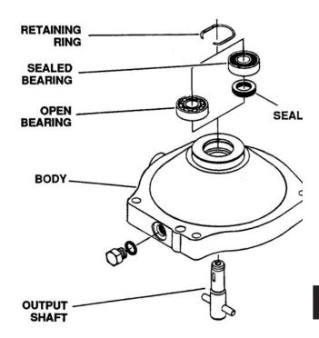
Figure 6-83. Removal of Output Bearing
