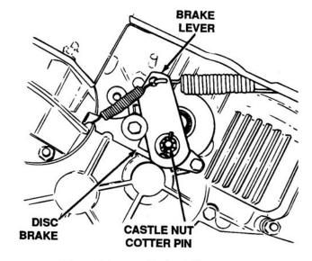
Figure 4-65. Brake Adjustment
