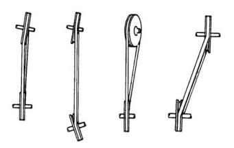
Figure 4-7. Pulley Misalignment
