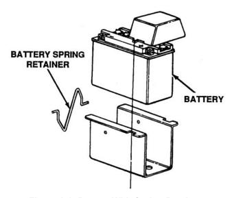
Figure 3-3. Battery With Spring Retainer.
