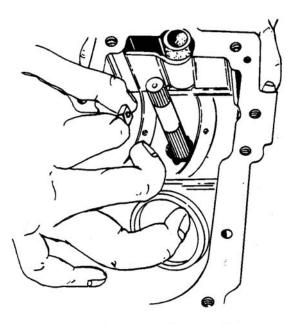
Figure 6-48. Installing Slot Guide
