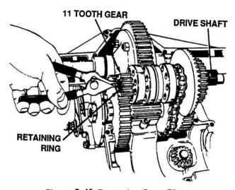
Figure 5-40. Removing Snap Ring
