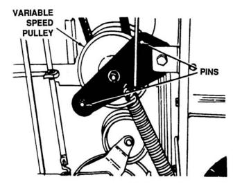
Figure 4-48. Variable Speed Pulley and Pins
