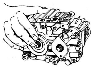
Figure 6-70. Positioning Transmission to Install Check Valve
