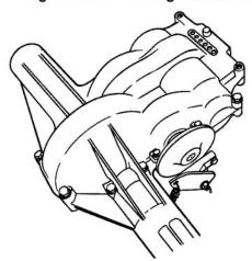
Figure 5-60. Securing Housing Halves Together
