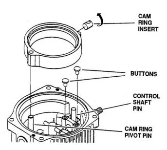
Figure 6-132. Cam Ring Installation
