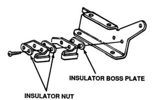
Figure 3-6. Safety Switch Insulator Nut Plates.
