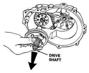
Figure 5-13. Removing Drive Shaft
