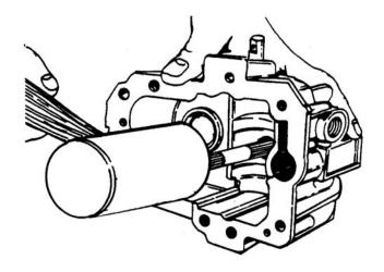
Figure 6-27. Removal of Pump Shaft
