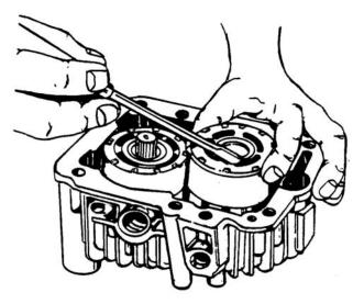
Figure 6-57. Positioning Piston Springs
