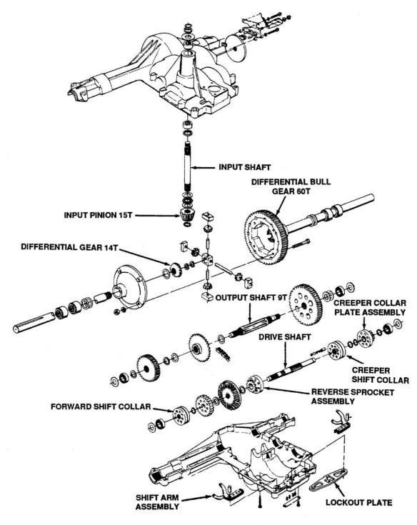
Figure 5-29. Two Speed Transaxle 717-1150
