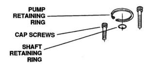
Figure 6-105. Removing Retaining Rings and Cap Screws
