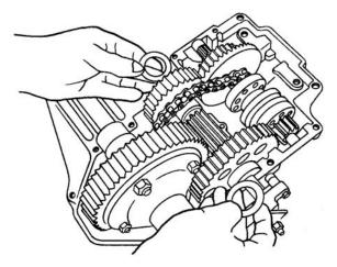
Figure 5-53. Placing Bearings Without Shims
