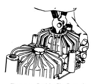
Figure 6-24. Retaining Ring Removal
