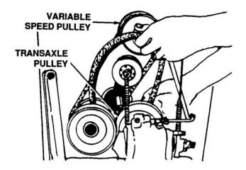
Figure 4-21. Location of V-Belt Pulleys
