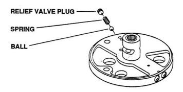
Figure 6-89. Removing Relief Valve Plug Spring and Ball
