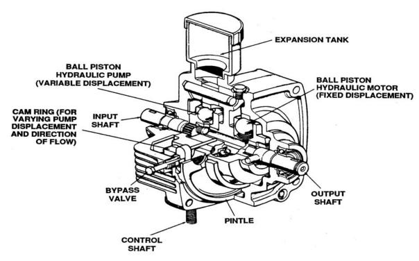
Figure 6-2. Model 7 Hydrostatic Transmission
