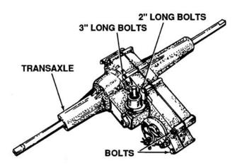
Figure 5-100. Pump Removal
