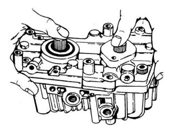
Figure 6-62. Installing Center Section
