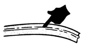
Figure 4-3. Belt Wear Due to Misalignment or Worn Pulley Groove
