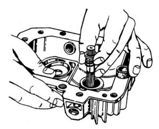
Figure 6-51. Installing Washer and Spring
