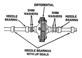
Figure 5-49. Location of Needle Bearings and Seals
