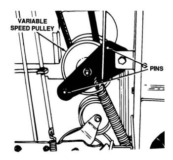
Figure 4-34. Location of Variable Speed Pulley and Pins
