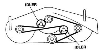
Figure 8-41. Belt Installation
