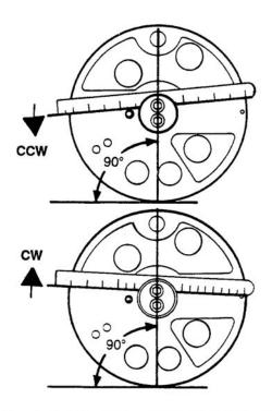
Figure 6-134. Determining Pintle Rotation
