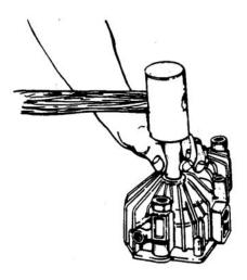
Figure 6-45. Pressing Seal Into Housing
