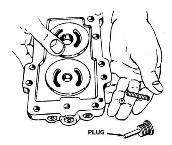
Figure 6-32. Ball and Spring Removal
