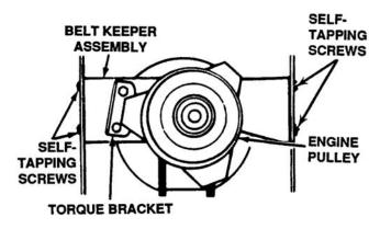
Figure 4-46. Removal of Torque Bracket
