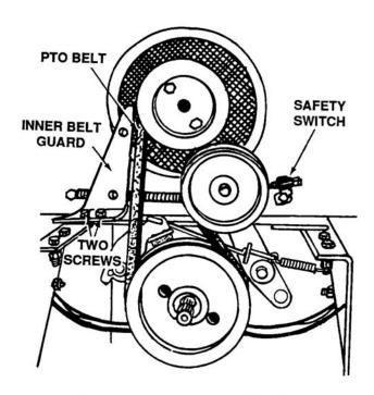
Figure 7-8. Removing PTO Belt
