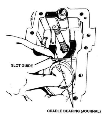
Figure 6-22. Removing Slot Guide and Cradle Bearings
