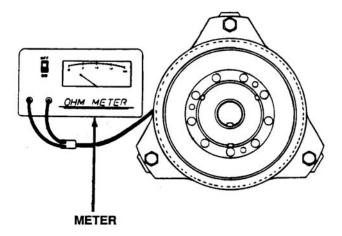
Figure 3-73. Measuring Clutch Coil Resistance
