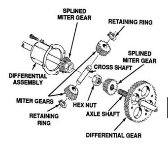
Figure 5-110. Differential Disassembly
