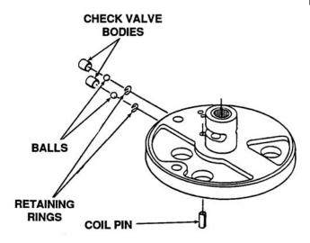
Figure 6-92. Removing Coil Pin
