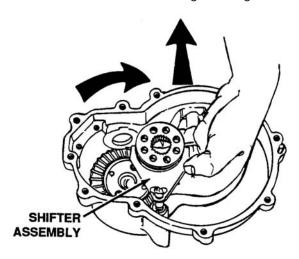
Figure 5-15. Removing Shifter Assembly
