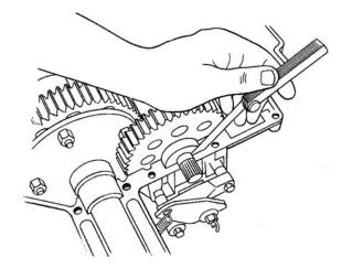
Figure 5-54. Checking for Shim Requirements
