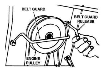
Figure 4-60. Releasing Belt Guard
