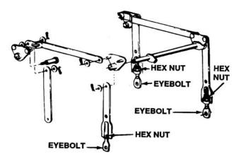
Figure 8-21. Deck Link Installation for 46-Inch Decks
