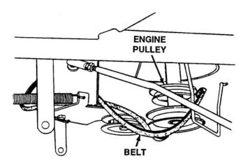
Figure 4-75. Belt Removal From Engine Pulley
