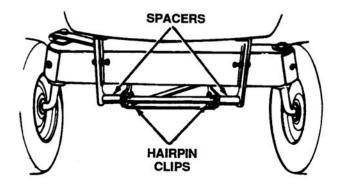
Figure 8-25. Disassembling Cross Bar
