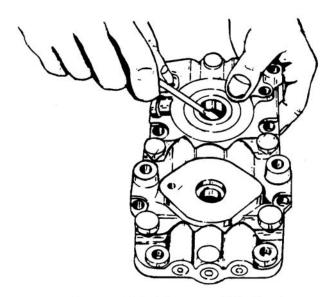
Figure 6-36. Removal of Oil Seal
