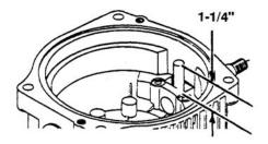
Figure 6-116. Install Dowel Pin
