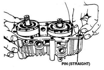
Figure 6-15. Removing Pins
