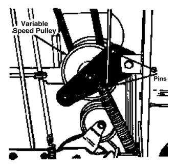
Figure 4-43. Belt Reassembly
