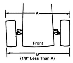
Figure 4-39. Units With Adjustable Tie Rods
