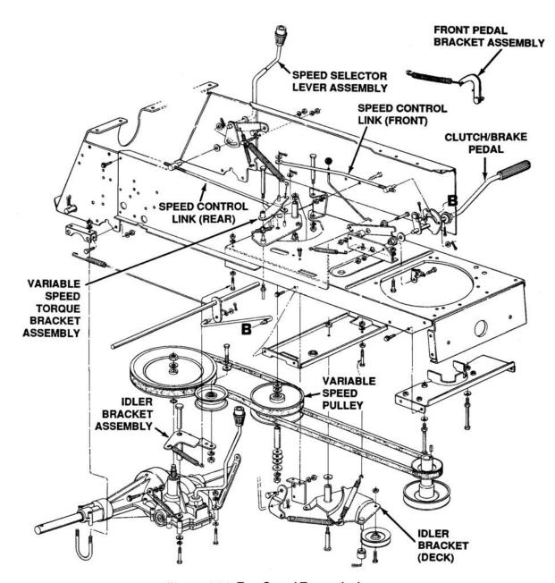
Figure 4-50. Two Speed Transmission
