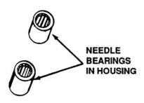
Figure 5 - 65. Needle Bearings
