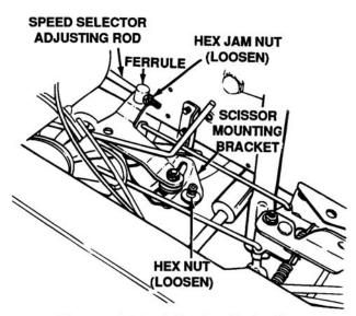
Figure 4-64. Adjusting Hydro-Gear Neutral Control
