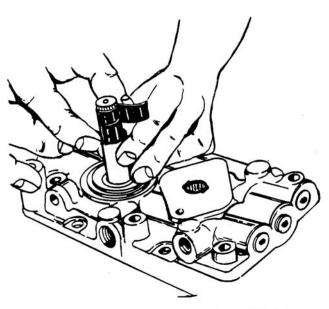
Figure 6-65. Covering Pump Shaft With Tape
