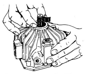
Figure 6-44. Covering Pump Shaft With Tape
