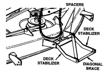
Figure 8-30. Deck Stabilizers and Diagonal Brace
