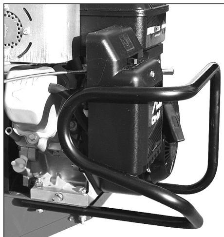
Figure 2: Loosely attach bumper to right side engine support bracket and base of engine. Tighten all four screws securely.
