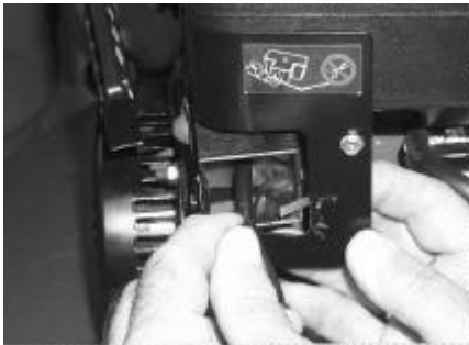
STEP D Push tie strap thru gap between starter switch box and tank skirt
