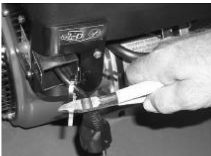
STEP J Push tab through catch and trim the end of the tab by one half inch
