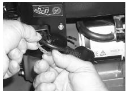
STEP I Loop second strap around plug cord and insert end into catch
