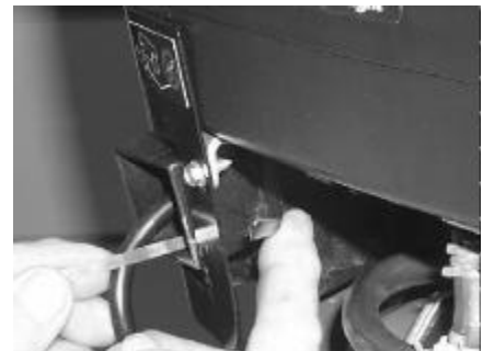
STEP C After tie strap insertion, loop tie strap
