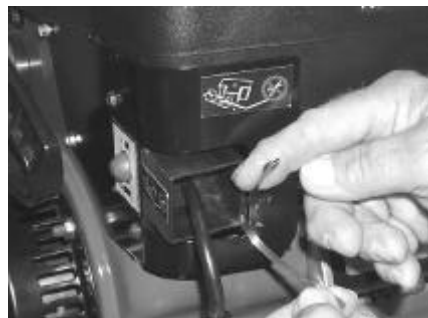
STEP H Insert second strap behind first strap on front right hand corner of starter switch box
