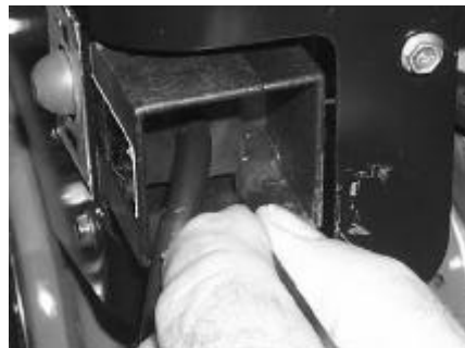
STEP B Insert tie strap into rear right or left hand corner as needed for proper cable position.
