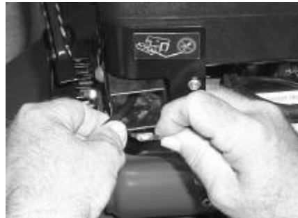
STEP E Insert tab in catch and push through
