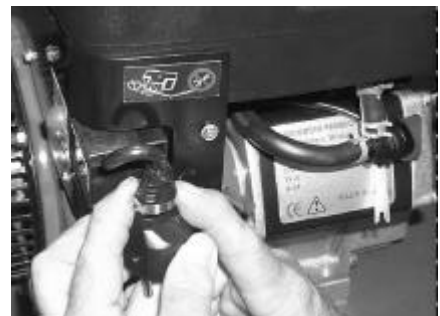
STEP L Hold plug end in position with connector body facing down
