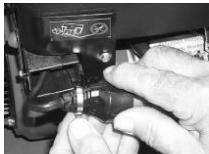
STEP K Position strap around plug as shown
