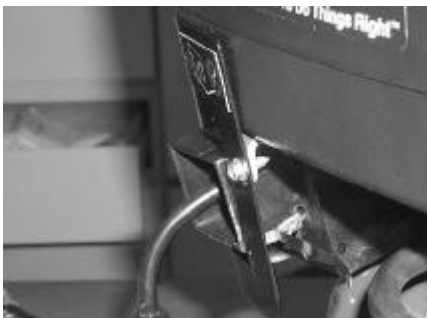
STEP G Push catch into gap between starter switch box and tank skirt
