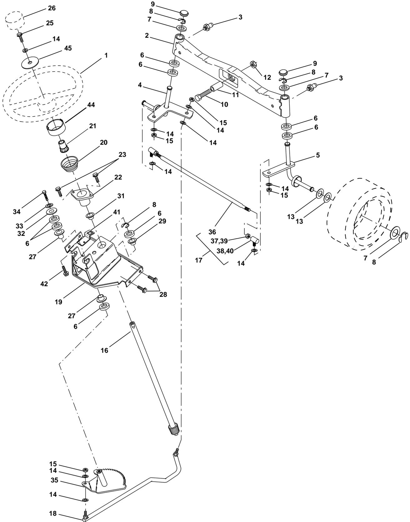
**PIÈCES DE RECHANGE****TRACTEUR - NUMÉRO DE MODÈLE PRGT2046B****ENSEMBLE DE LA DIRECTION**
