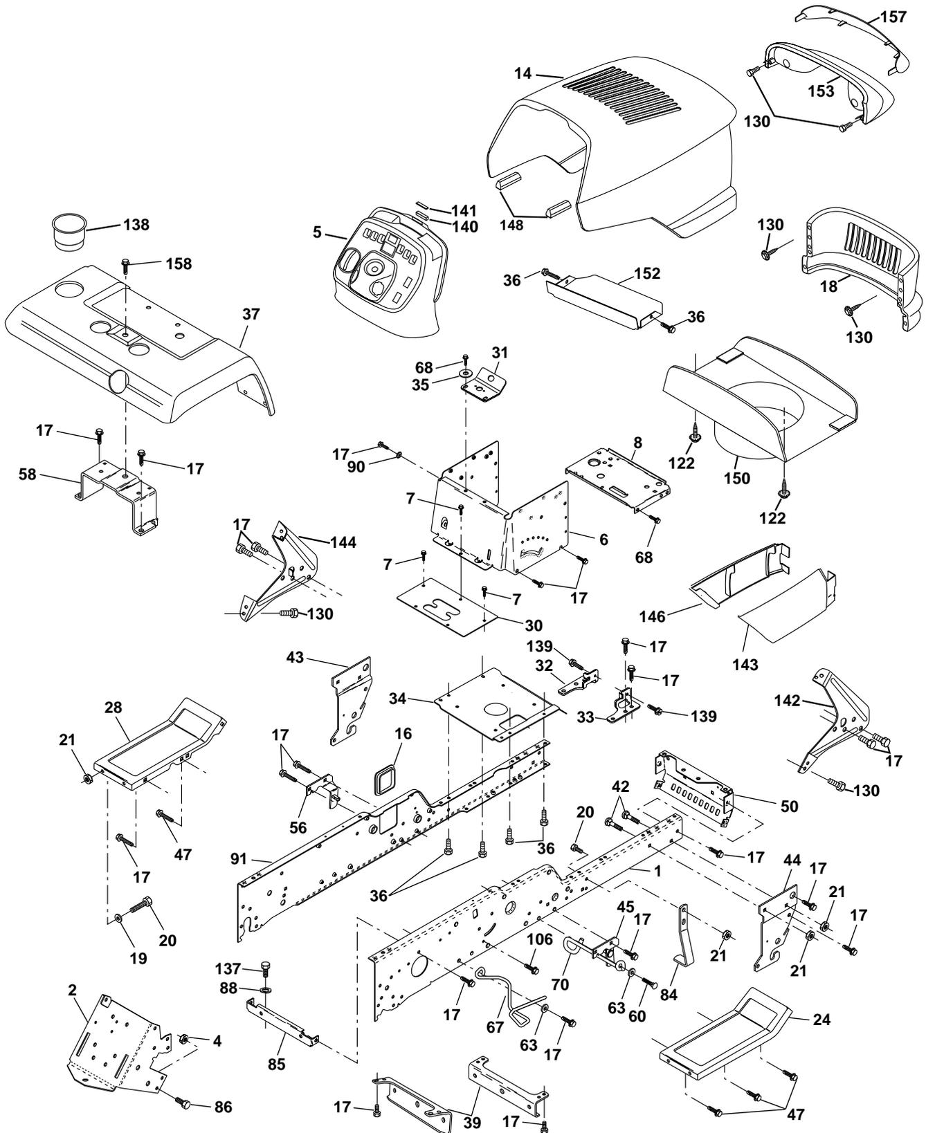
**PIÈCES DE RECHANGE****TRACTEUR - NUMÉRO DE MODÈLE PRGT2046B****CHÂSSIS ET LES ENCEINTES**
