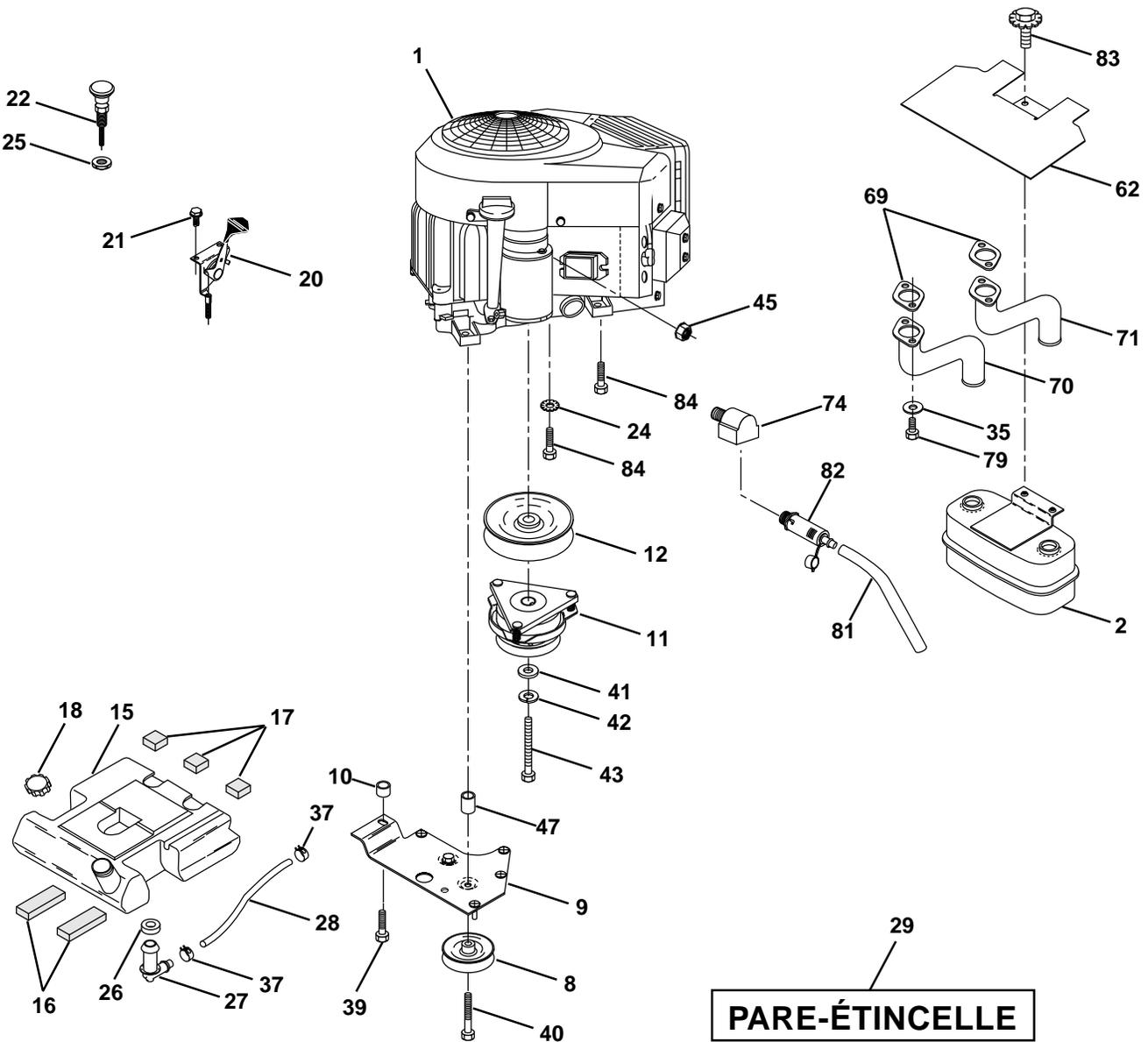
**PIÈCES DE RECHANGE****TRACTEUR - NUMÉRO DE MODÈLE PRGT2046B****MOTEUR**
