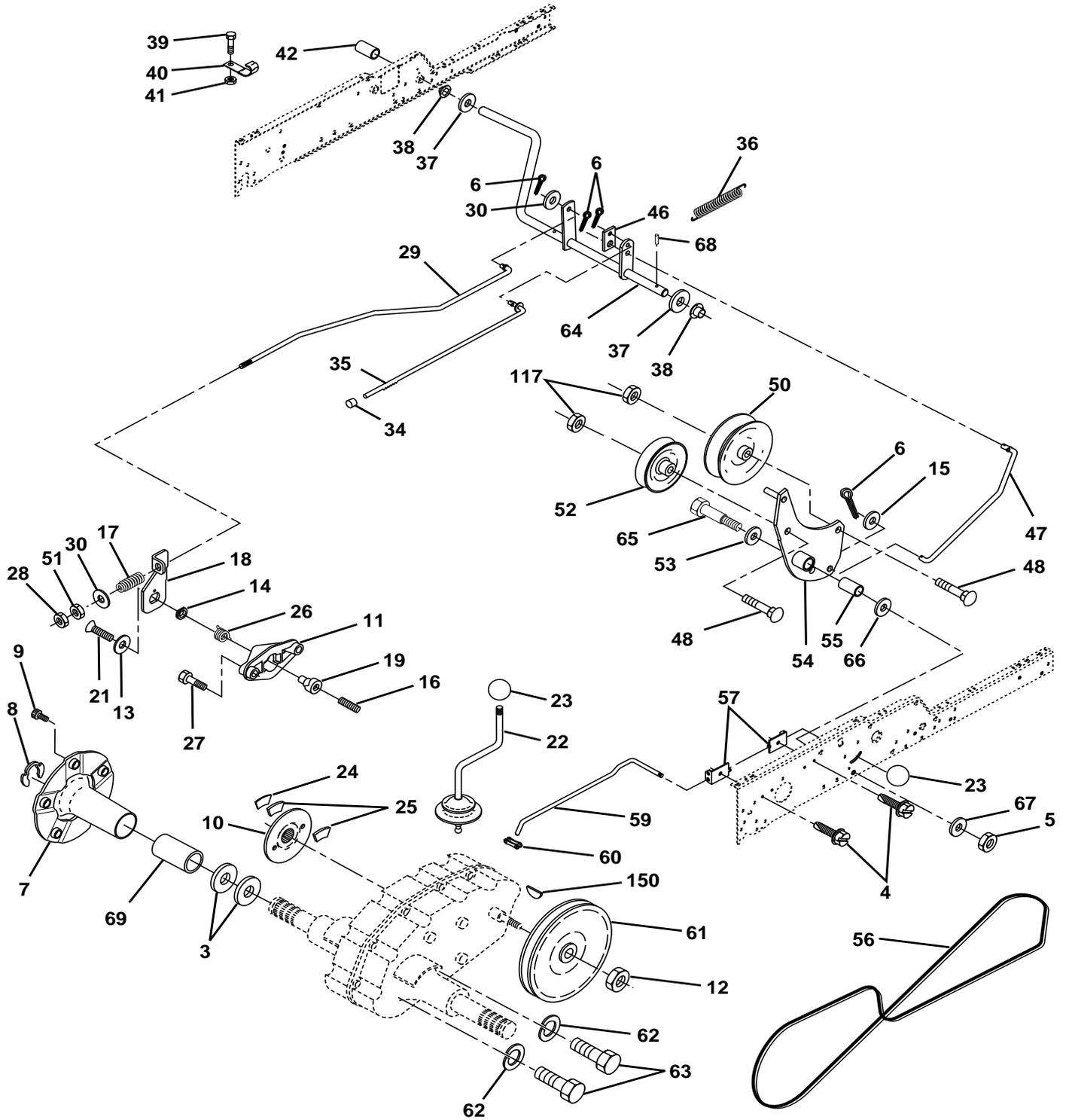
**PIÈCES DE RECHANGE****TRACTEUR - NUMÉRO DE MODÈLE PRGT2046B****ENTRAÎNEMENT**
