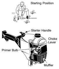
**A WARNING:** The trimmer head will turn while starting the engine. Avoid any contact with the muffler. A hot muffler can cause serious burns.
