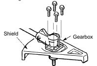
· Insert and thread the 4 mounting screws through the holes of the gearbox and the metal shield. Tighten evenly and securely with the hex wrench provided.
