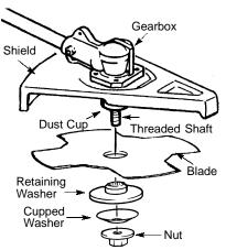
**NOTE:** Make sure all parts are in place as illustrated, and the blade is sandwiched between the dust cup and the retaining washer. There should be no space between the blade and the dust cup or the retaining washer. 6
