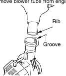
Insert the elbow tube into the blower outlet. Make sure elbow tube rib is aligned with the blower outlet groove.
