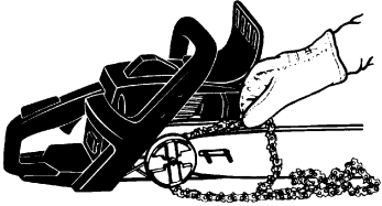
Place chain onto the sprocket
