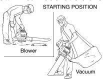
**WARNING:** When starting engine, hold the unit as illustrated. Do not set unit on any surface except a clean, hard area when starting engine or while engine is running. Debris such as gravel, sand, dust, grass, etc. could be picked up by the air intake and thrown out through the discharge opening, damaging the unit or property, or causing serious injury to bystanders or the operator.
