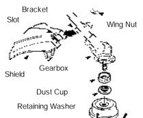
**NOTE:** Make sure all parts are properly installed as illustrated in the illustration before installing the trimmer head.
