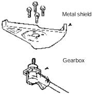
**S** Insert the 4 mounting screws through the bottom of the shield. Thread them into the gearbox. Tighten evenly and securely with one of the hex wrenches provided.
