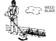
NOTE: If your unit has been assembled for trimmerheaduse, refertothesectionATTACH-ING THE PLASTIC SHIELD ANDTRIMMER HEAD and reverse the steps to remove the plastic shield and trimmer head before you mount the metal shield and blade. Store these partsforful treuse. Neveruse the trimmerhead with the metal blade installed.
