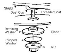
WARNING: Do not use any blades, or fastening hardware other than the washersandnutsillustrated.Thesepartsmust be provided by Weed Eater, and installed as
