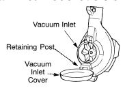
Place the hooks on the vacuum tube on the retaining posts; pivot tube into position. Secure vacuum tube by turning the knob clockwise until tight.
