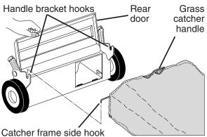
DOOR PIVOT PIN MOUNTED Pivot pins Rear Grass door catcher handle Catcher frame hook DOOR SLOT MOUNTED Rear door slots Grass catcher handle
