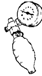
PN 215432-01 Pressure Test Tool
