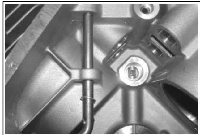
Figure 11-5. Installing 8 mm Governor Cross Shaft.
