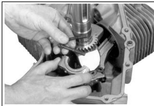
Figure 9-66. Mark End Cap with Cylinder Number Before Removal.
