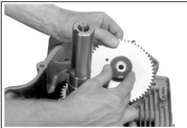
Figure 11-15. Change Shim to Obtain Correct End Play.
