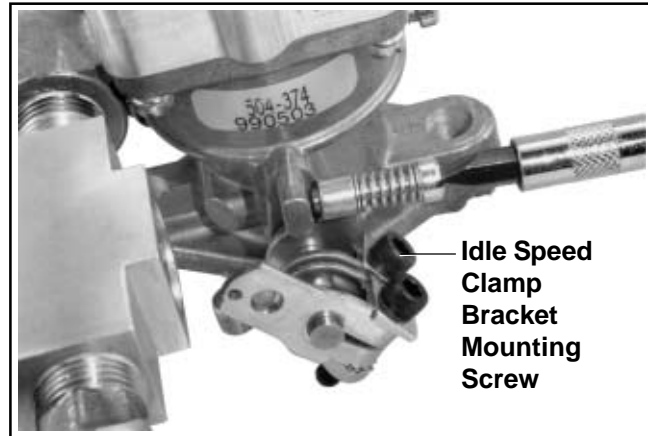
Figure 5A-8. Backing Off Idle Speed Screw.
