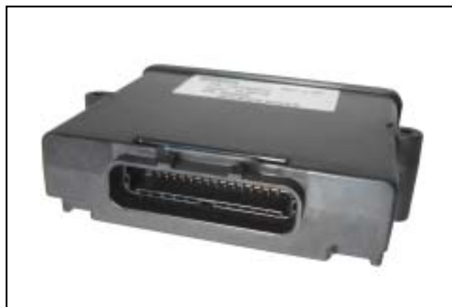
Figure 5B-3. “32 Pin” (MSE 1.1) Plastic-Cased ECU.
