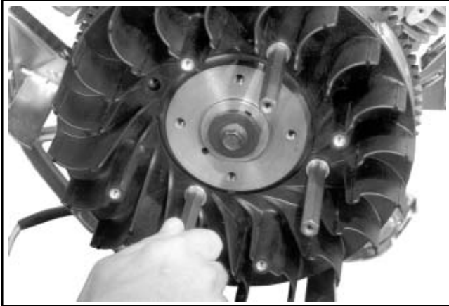
Figure 11-32. Installing Supports for Metal Grass Screen.
