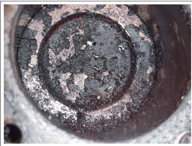
Figure 100. Carbon – Due to what?
