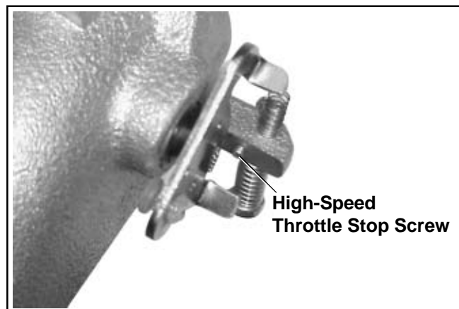
Figure 5B-38. Throttle Details.
