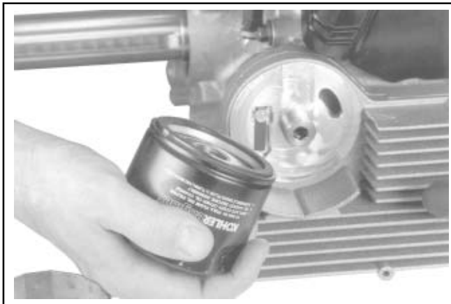
Figure 11-93. Installing New Oil Filter.
