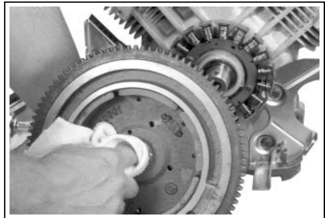
Figure 11-27. Clean and Dry Flywheel Hub.
