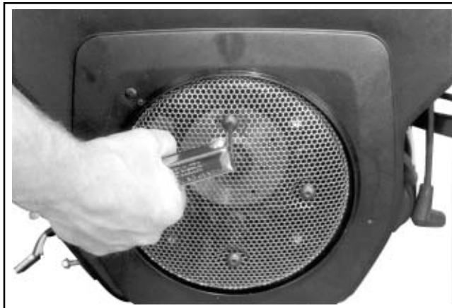
Figure 9-32. Removing Metal Grass Screen.
