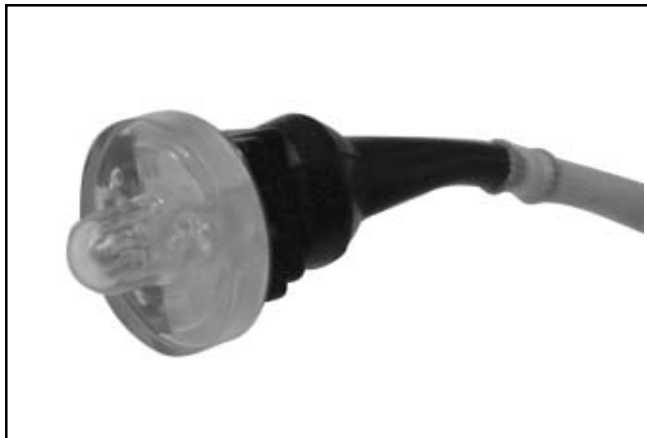
Figure 5B-20. Volt Test Light.
