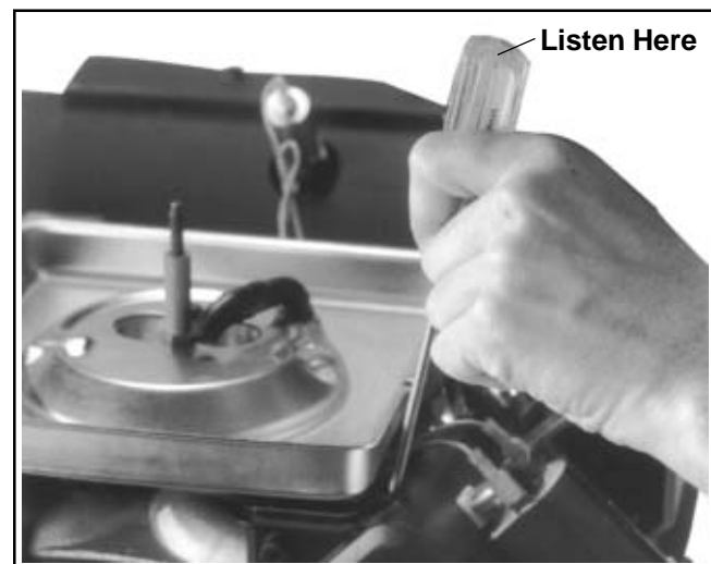
Figure 5B-19. Checking Injectors.
