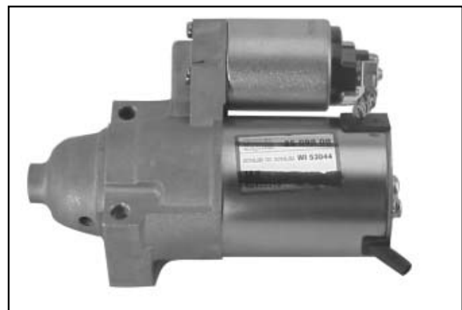
Figure 8-40. Completed Delco-Remy Starter.
