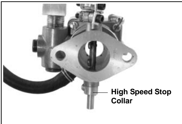
Figure 5A-11. Full Throttle Position.
