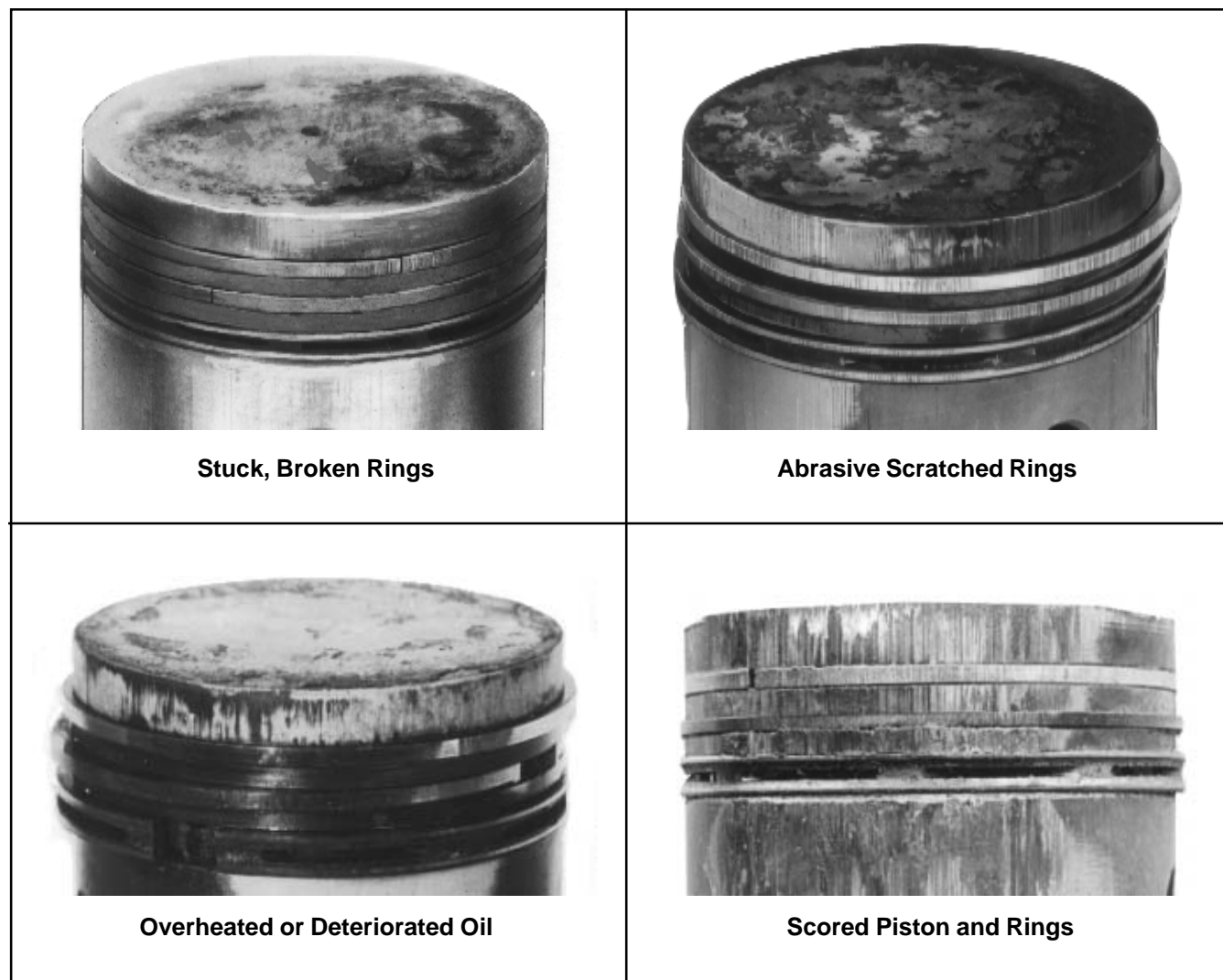
Figure 10-8. Common Types of Piston Damage.
