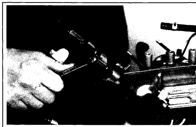
Figure 9-22. Removing #2 Side Valve Cover Studs.
