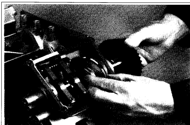
Figure 11-28. Installing Camshaft Through Governor.
