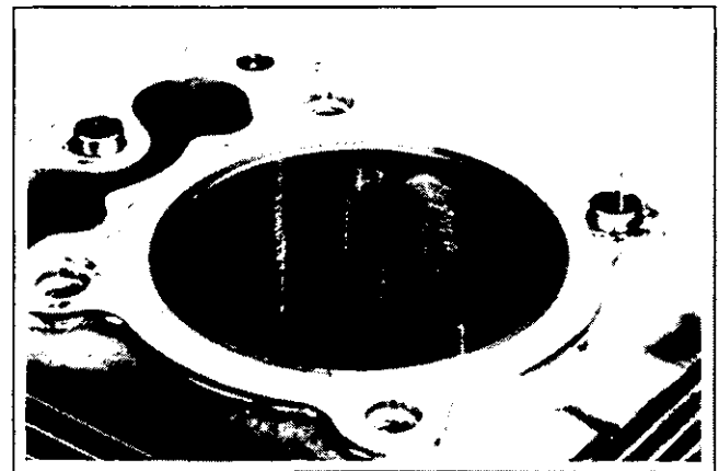
Figure 10–2. Cylinder Bore Crosshatch After Honing.
