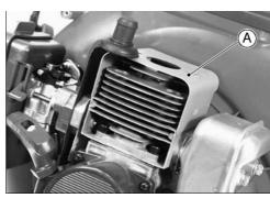
Remove: Air Filter Cap [A] Air Filter Element [B]
