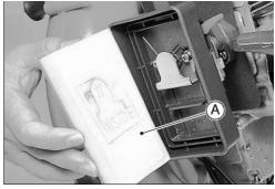
• Install the air filter cap [A] first its lower end [B], and then upper end firmly.
