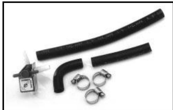
During the winter of 1996-97, we received some reports of icing in the breather hose on CV18-25 engines. A new anti-icing kit, 71/501 54-755-17 has been developed to alleviate the problem. The kit includes a manual, two way valve for rerouting the breather in cold weather.
