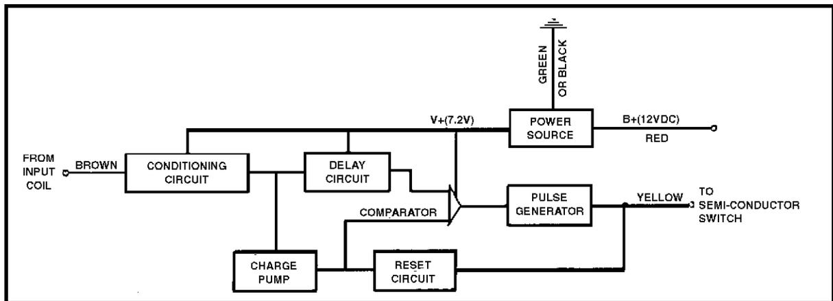
**Figure 4. Block Diagram - Spark Advance Module.**
