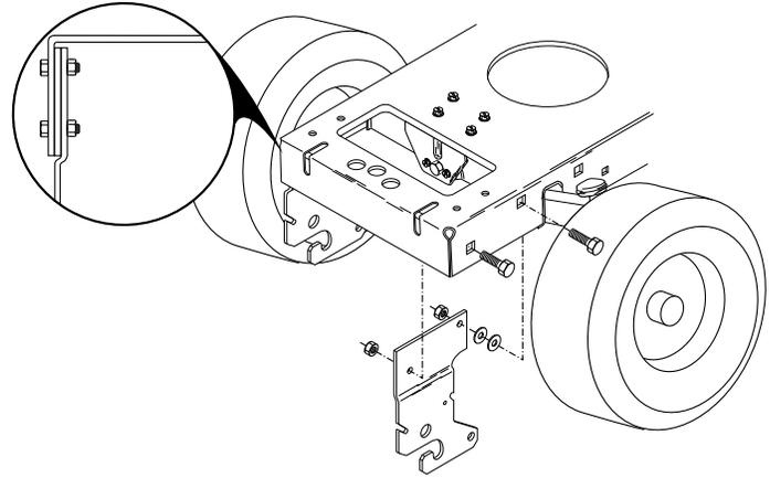
1. LT. tractors - the tractor clutch pedal gets hung up halfway and will not release, causing customer to pull foot pedal back with his toe of shoe to engage drive belt - Solution - drop the tractor motion drive clutch idler assembly and lubricate the idler pin with grease. If the welded pin is rust pitted, you can replace with clutch bracket kit 71/917 #137329
