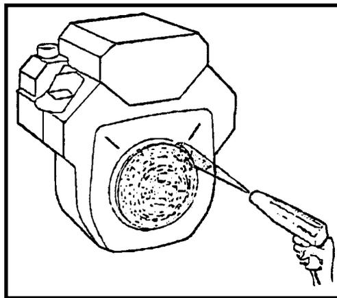
4. The marks you made on the blower housing, corresponding to the firing points of the cylinders, should be 90° apart. As you accelerated, the timing should have advanced 5 to 15, and the line on the screen should have moved 1/2" to 3/4" (13-16 mm) counter clockwise from the mark on the blower housing.
