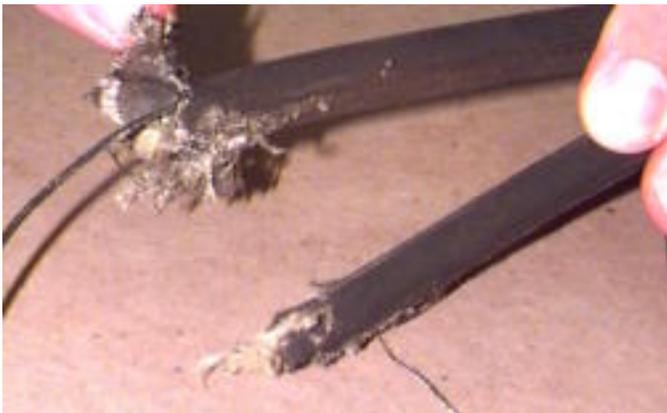
**Shock Load fracture of V-belt**
