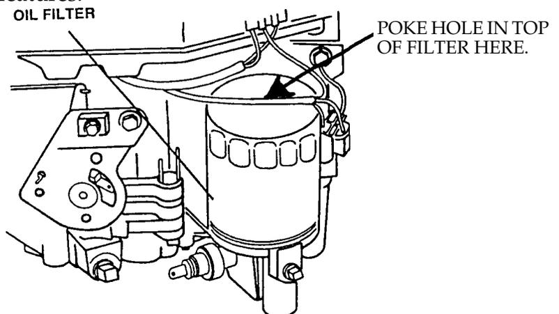
PREVENT OIL FROM SPILLING ALL OVER THE WHEN CHANGING FILTER. POKING A HOLE IN THE TOP OF THE FILTER WILL VENT SYSTEM AND ALLOW OIL TO DRAIN OUT THROUGH ENGINE SUMP.
