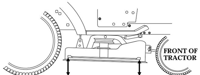
**SET RAKE AT 1/8" TO 1/2" WITH OPTIMUM SETTING AT 1/4". NOTE: EXCESSIVE DECK RAKE MAY CAUSE PREMATURE BELT FAILURE. ALWAYS CHECK DECK RAKE WHEN REPLACING THE MOWER DRIVE BELT OR WHEN LEVELING THE DECK.**
