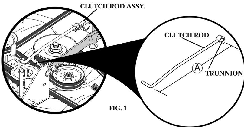
To loosen a tight belt turn the clutch rod trunion in clockwise.
