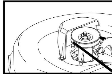
**CAUTION:** Do not allow the customer to operate a mower with any Mandrel safety guards removed.
