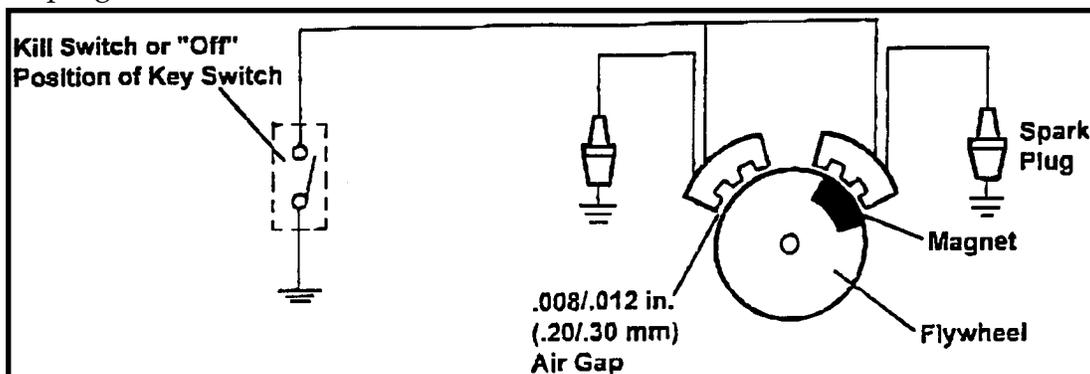
**Figure 1. Capacitive Discharge Ignition System.**
