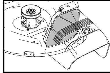
**CAUTION:** Do not allow the customer to operate the mower with the safety discharge guard removed.
