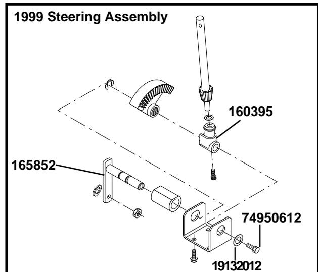
At the end of the pittman shaft, a bolt and washer replace the clip ring.
