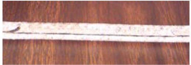
**V-belt Cut from installation by Prying v-belt over pulley** Replace v-belt with correct installation procedure.
