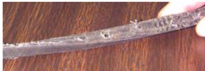
**V-belt Abrasion from idler locked up** The v-belt will be worn across the width of the belt. The material will be carbonized and show cracks.
