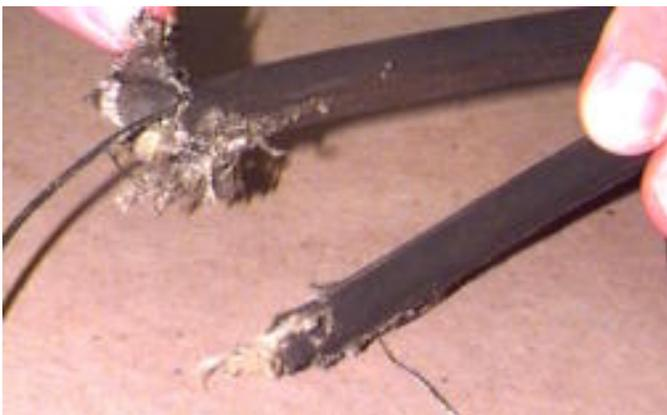
**Shock Load fracture of V-belt**
