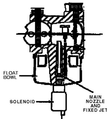
This type of Anti-Afterfire system works by shutting off fuel flow through the main jet. The solenoid is energized when the ignition switch is turned to the on position, when the switch is turned to the off position the spring loaded plunger is pushed into the jet. This system works best when the throttle control is in the mid to full position. This reduces the amount of fuel in the idle circuit of the carburetor. Very little fuel will be available to burn in the muffler and afterfire.
