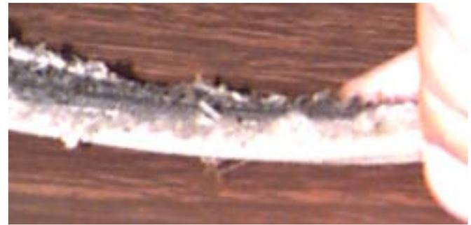
**V-belt bottoms out in Pulley or Wear from rough Pulley** V-belt worn away at the sides of the 'v'. Check pulley groove and v-belt width. Also check the v-belt pulleys or small rock wedged into the pulley. Worn v-belt sidewalls, v-belt rides at bottom of the pulley groove, replace v-belt and replace damaged 'V' pulley. The pulley groove should not be rough, rusty, or worn.
