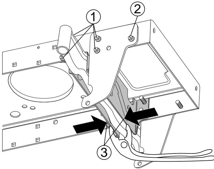
1. LOOSEN FOUR BOLTS HOLDING THE FRONT AXLE BRACES ON RIGHT HAND SIDE OF THE TRACTOR, (ITEM 1), DO NOT LOOSEN BOLT, (ITEM 2).
