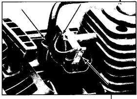
5. If there is still no spark, check the ignition connection leads and contacts for poor connections, dirt, breakage or damaged installation. Check ignition module air gap, it should be set from .012 to .015 in.
