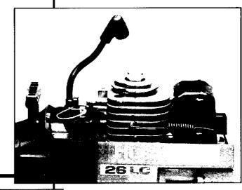
Remove throttle wire from throttle trigger assembly.
