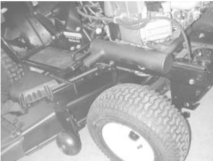
GARDEN TRACTORS BEFORE 2001 HAD THE MUFFLER BESIDE THE ENGINE
