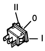
The switch is off in position "0" supplies current to the handle heater in position "I"
