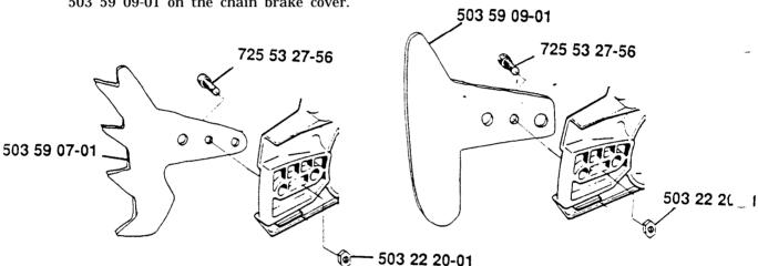
**NOTE!** Both inner and outer spike must be mounted.
