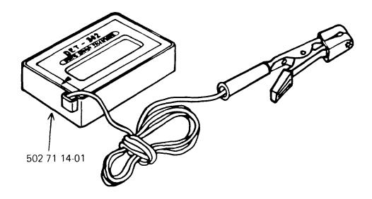
The tachometer, which is in "pocket size" (40 x 60 x 15 mm) is used in the following way:
