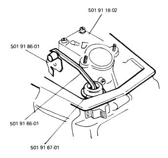
The carburettor Ref. No. 501 91 18-01 will not be available as a spare part. When mounting the carburettor Ref. No. 501 91 18-02 on the model 181, the throttle shaft Ref. No. 501 81 44-01 must be ordered separately.
