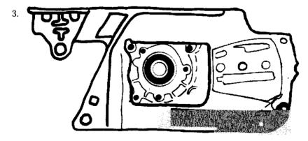
Put the repair part on the crankcase, guided in the front by the crankcase screw and at the back along the crankcase.
