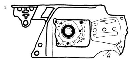
Cut away material in the front (A) along the plane to the removed crankcase screw.
