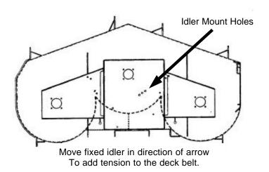
To add tension, remove the deck belt; remove the thin fixed idler, and move it left and rearward by one hole location. Reinstall the mower deck belt.
