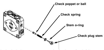
Install the new shock valve in the same sequence, noting that the small end of the new spring goes into the .031 poppet, and the check plug stem is replaced by a hex head housing containing a new o-ring. Torque shock valves to 180 - 240 in. lbs. (14-20 N.m). Repeat instructions on the left pump.
