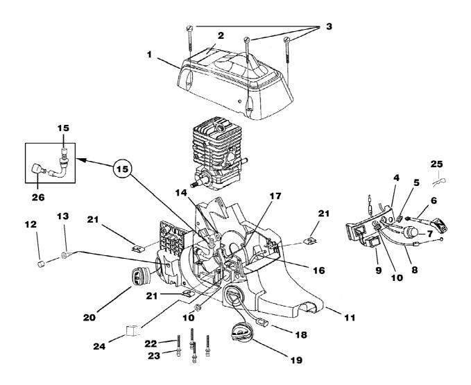
z3850bc Chain Saw UT-10773 Engine Housing - Fuel Tank - Oil Tank Page 8 of 14
