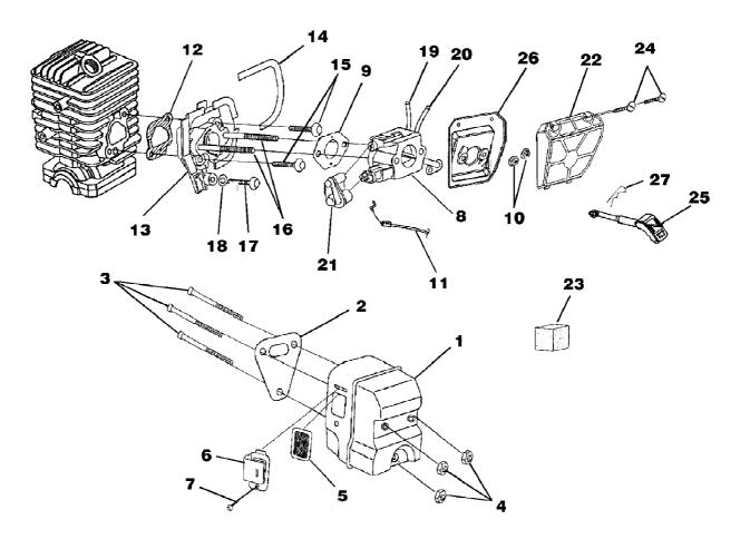
z3850bc Chain Saw UT-10773 Carburetor - Muffler - Air Filter Page 4 of 14
