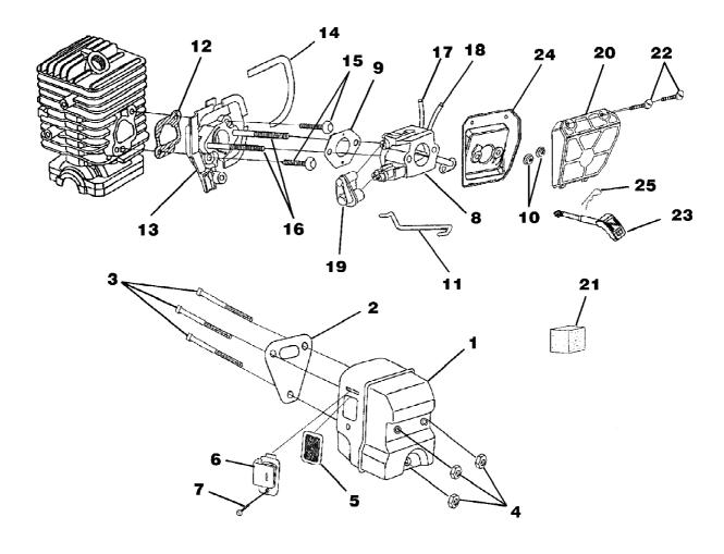
z3300c Chain Saw UT-10809 Carburetor - Muffler - Air Filter Page 4 of 14
