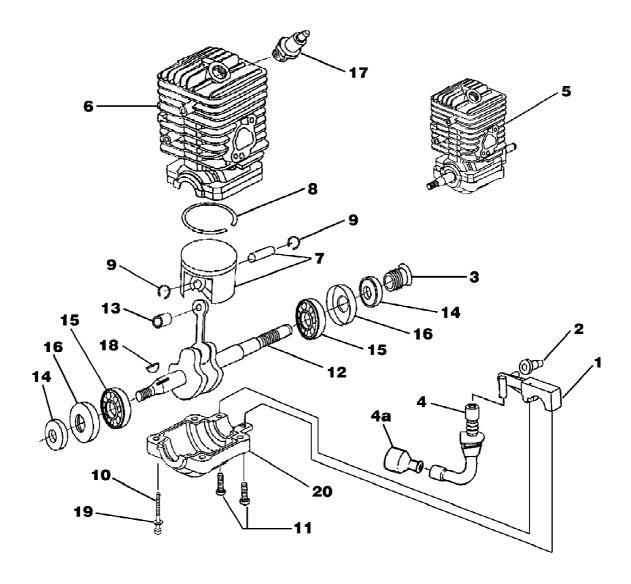
z3300c Chain Saw UT-10786 Engine Internal - Oil Pump Page 10 of 14
