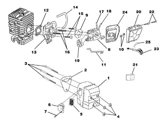
n3014 w/cc Chain Saw UT-10933 Carburetor - Muffler - Air Filter Page 4 of 14
