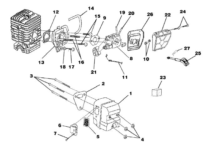
i4550b Chain Saw UT-10807 Carburetor - Muffler - Air Filter Page 4 of 14
