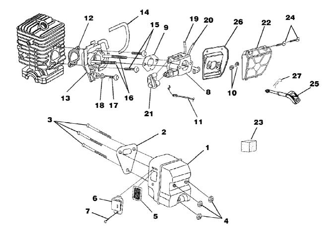
i4150b Chain Saw UT-10839 Carburetor - Muffler - Air Filter Page 4 of 14
