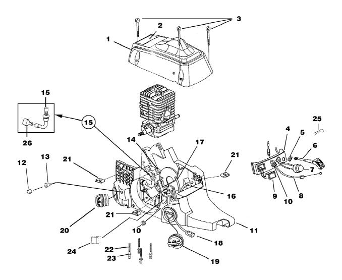
i4150b Chain Saw UT-10808 Engine Housing - Fuel Tank - Oil Tank Page 8 of 14
