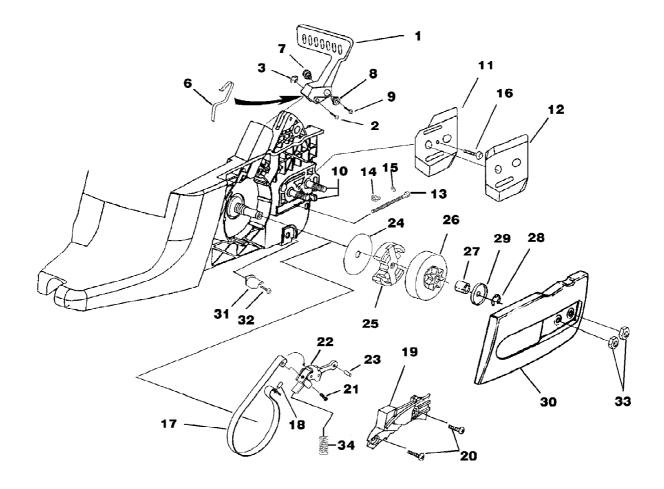
i4150b Chain Saw UT-10808 Clutch - Chain Brake - Drive Case Cover Page 6 of 14
