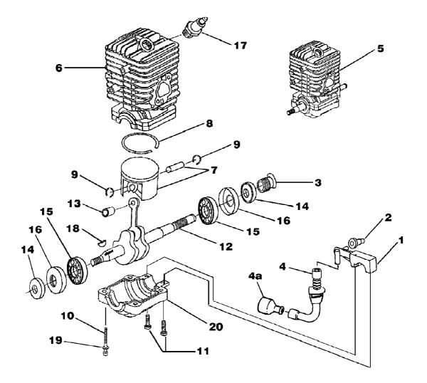
i4150b Chain Saw UT-10808 Engine Internal - Oil Pump Page 10 of 14
