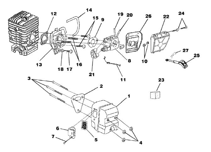
i4150b Chain Saw UT-10808 Carburetor - Muffler - Air Filter Page 4 of 14
