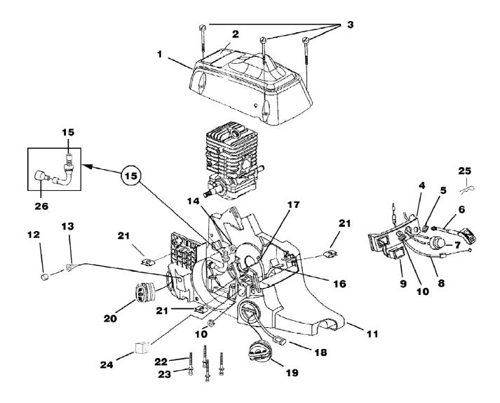
i3850b Chain Saw UT-10869 Engine Housing - Fuel Tank - Oil Tank Page 8 of 14
