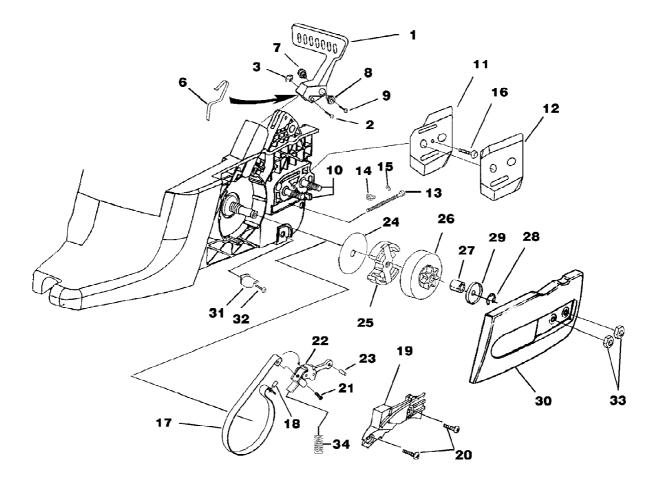
i3350b Chain Saw UT-10840 Clutch - Chain Brake - Drive Case Cover Page 6 of 14
