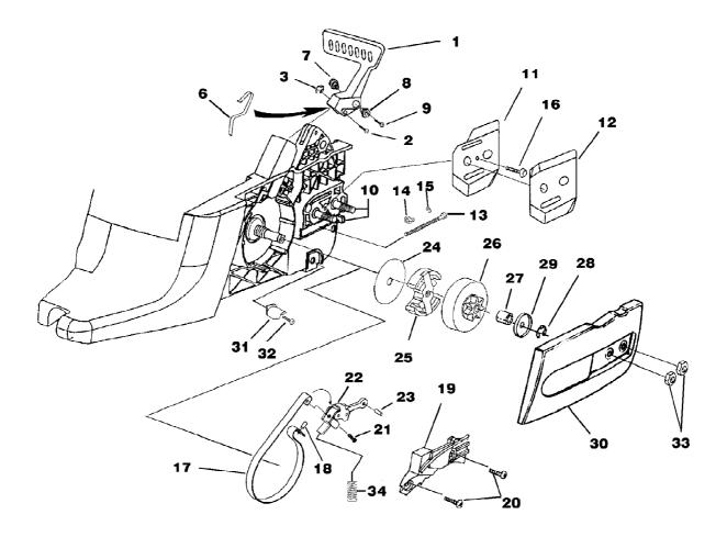
d4550bc Chain Saw UT-10836 Clutch - Chain Brake - Drive Case Cover Page 6 of 14
