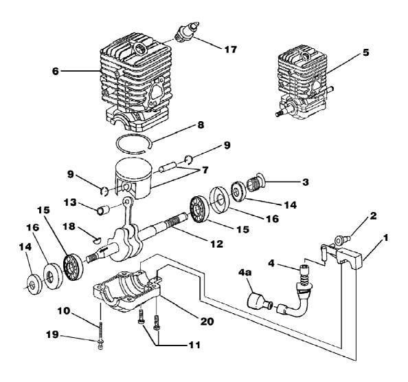
d4550bc Chain Saw UT-10836 Engine Internal - Oil Pump Page 10 of 14
