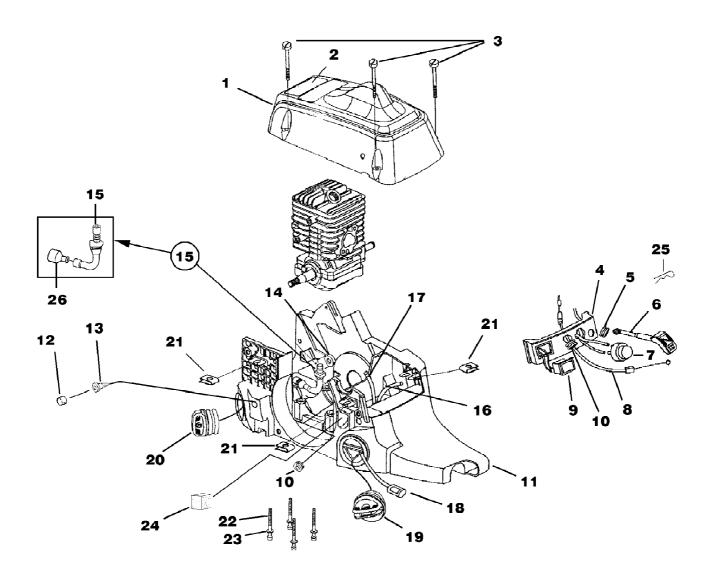
d3850bc Chain Saw UT-10865 Engine Housing - Fuel Tank - Oil Tank Page 8 of 14
