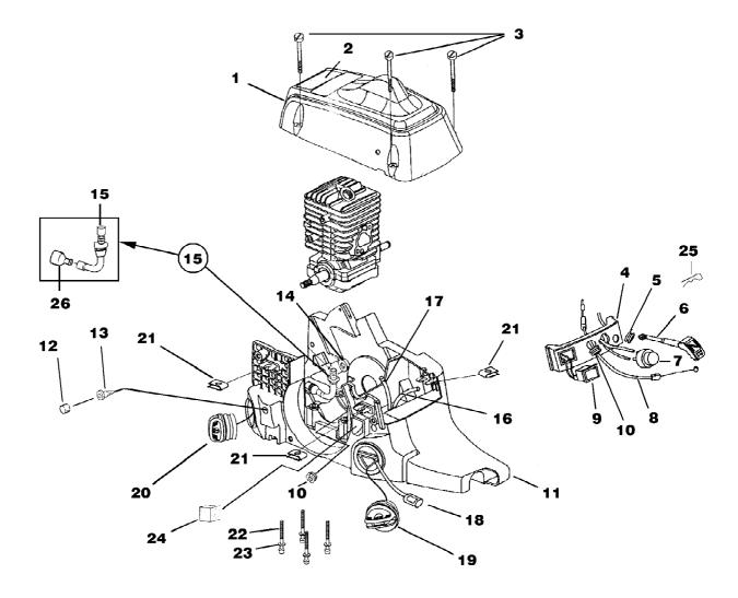
d3850bc Chain Saw UT-10770-A Engine Housing - Fuel Tank - Oil Tank
