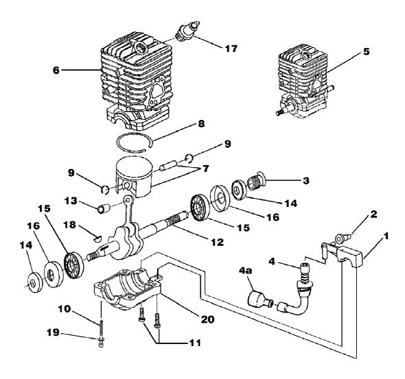
d3850bc Chain Saw UT-10770-A Engine Internal - Oil Pump Page 10 of 14
