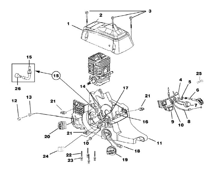
d3850b Chain Saw UT-10886 Engine Housing - Fuel Tank - Oil Tank
