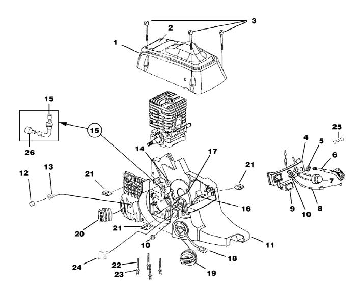
d3850b Chain Saw UT-10861 Engine Housing - Fuel Tank - Oil Tank
