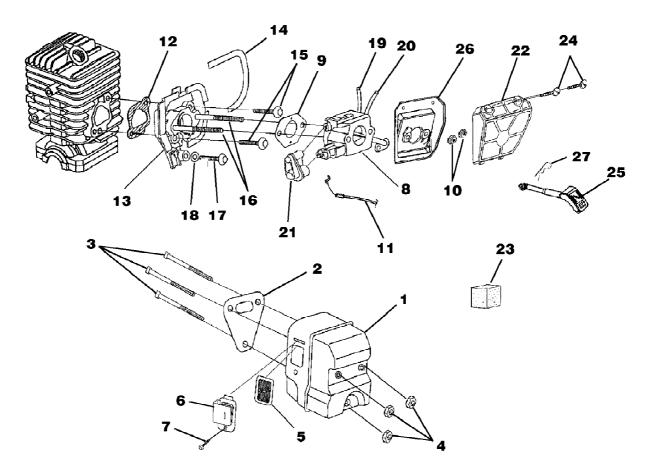
d3850b Chain Saw UT-10861 Carburetor - Muffler - Air Filter Page 4 of 14
