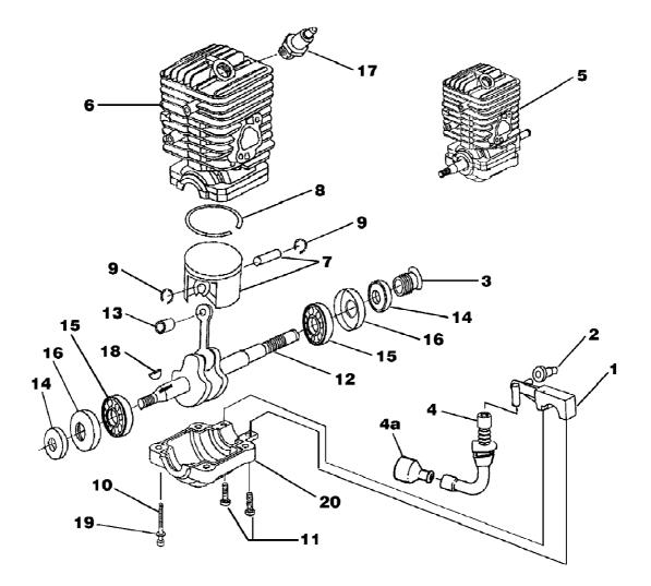
d3850b Chain Saw UT-10769-A Engine Internal - Oil Pump Page 10 of 14
