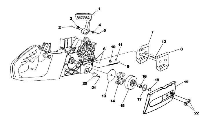
d3800c Chain Saw UT-10783 Clutch - Hand Guard - Drive Case Cover Page 6 of 14
