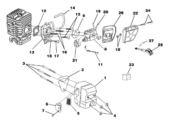
d3350b Chain Saw UT-10767 Carburetor - Muffler - Air Filter Page 4 of 14
