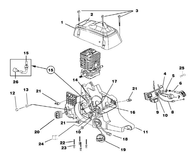
d3350b Chain Saw UT-10767 Engine Housing - Fuel Tank - Oil Tank Page 8 of 14
