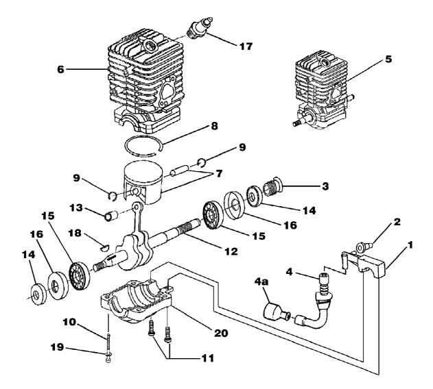
d3300c Chain Saw UT-10784-A Engine Internal - Oil Pump Page 10 of 14
