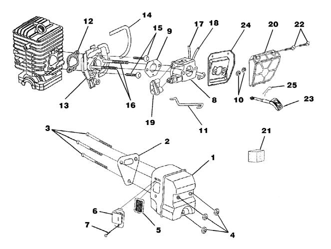
d3300c Chain Saw UT-10784-A Carburetor - Muffler - Air Filter Page 4 of 14
