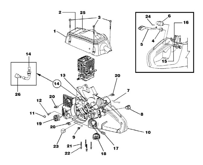
d3300c Chain Saw UT-10784-A Engine Housing - Fuel Tank - Oil Tank
