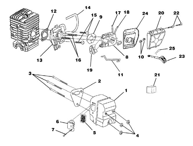
d3300 Chain Saw UT-10821 Carburetor - Muffler - Air Filter Page 4 of 14
