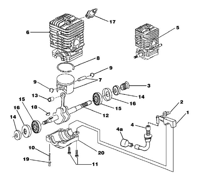
d3300 Chain Saw UT-10779 Engine Internal - Oil Pump Page 10 of 14
