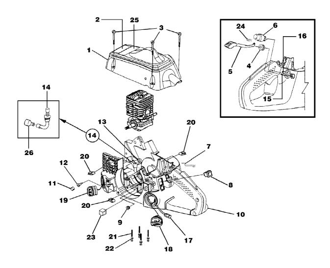
d3300 Chain Saw UT-10779 Engine Housing - Fuel Tank - Oil Tank Page 8 of 14
