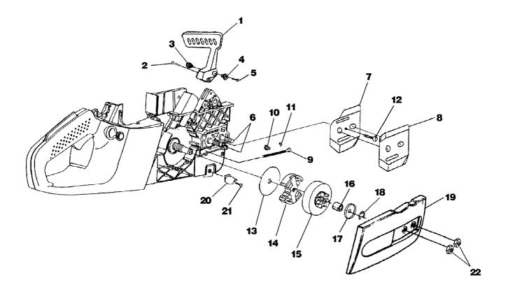
d3300 Chain Saw UT-10779 Clutch - Hand Guard - Drive Case Cover Page 6 of 14
