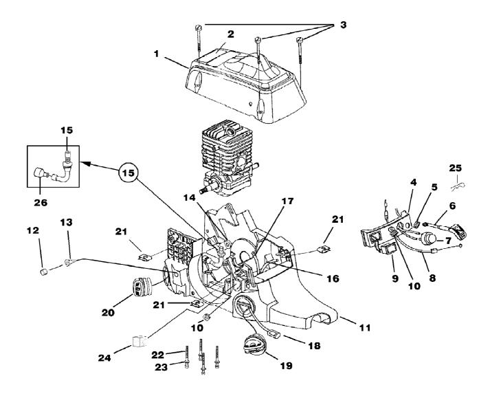
Timberman 45 cc 18" Chain Saw UT-10910 Engine Housing - Fuel Tank - Oil Tank Page 8 of 14
