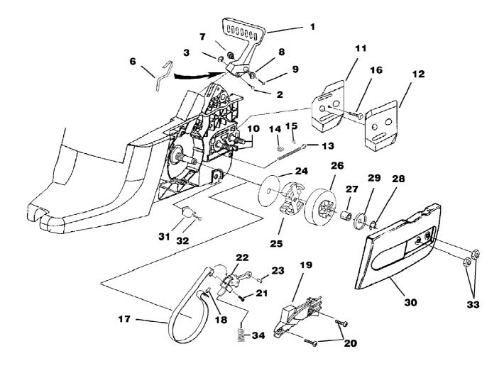
Timberman 45 cc 18" Chain Saw UT-10910 Clutch - Chain Brake - Drive Case Cover Page 6 of 14
