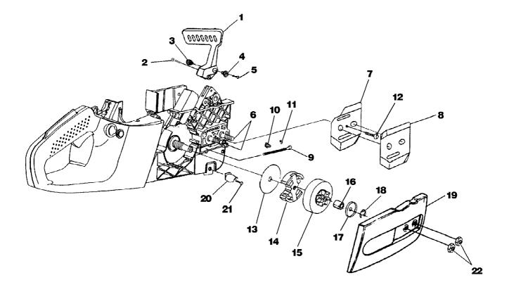
PS33 Chain Saw UT-10819 Clutch - Hand Guard - Drive Case Cover Page 6 of 14
