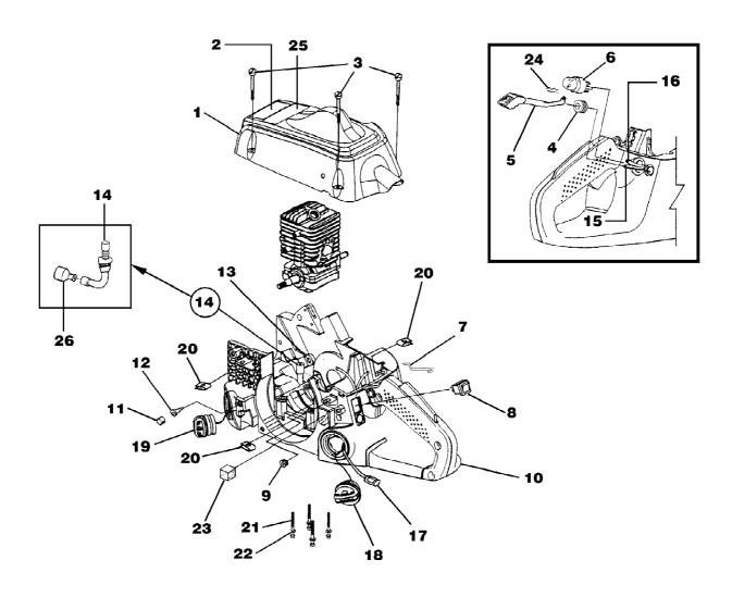
N3014 Chain Saw UT-10799-R Engine Housing - Fuel Tank - Oil Tank Page 8 of 14
